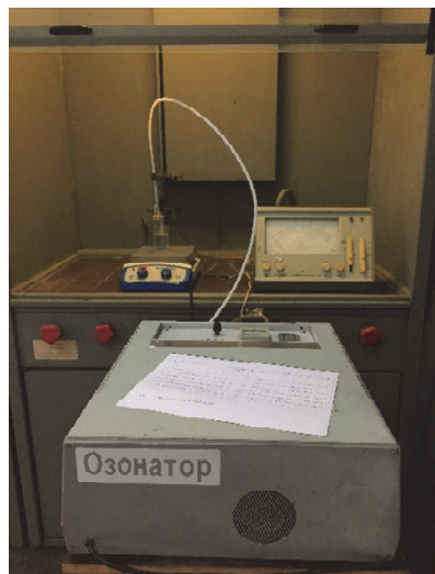
Figure 1 Ozone generator with redox-potential control system in ores samples oxidizing media
