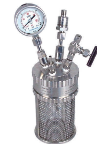
Figure 3 Laboratory autoclave with oxygen supply to the chamber and pressure up to 1.5 MPa
