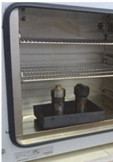
Figure 2 0.15 dm 3 sealed vessels with Teflon inserts without pressure control
