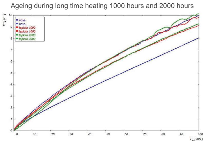
**Figure 9** Indentation curves measured before and after action higher temperature on surface of sample of polymer material
