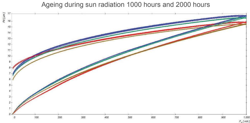
**Figure 8** Indentation curves measured before and after action sun radiation on surface of sample of polymer material
