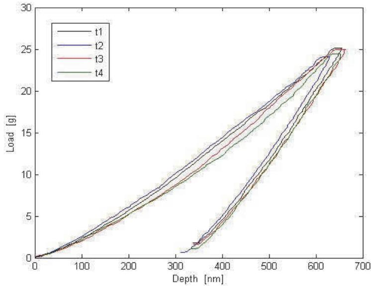
**Figure 4** Indentation curves with maximal load 25 g
