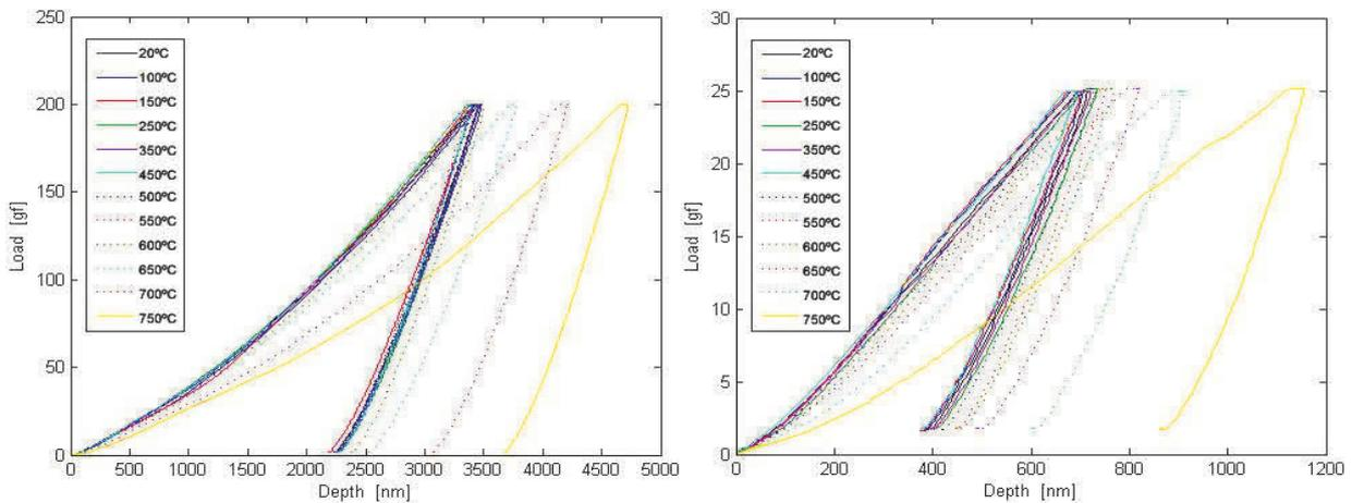
**Figure 6** Comparison of indentation curves with maximal load 200g and 25g on sample after temperature loading from 20 C to 750 C
