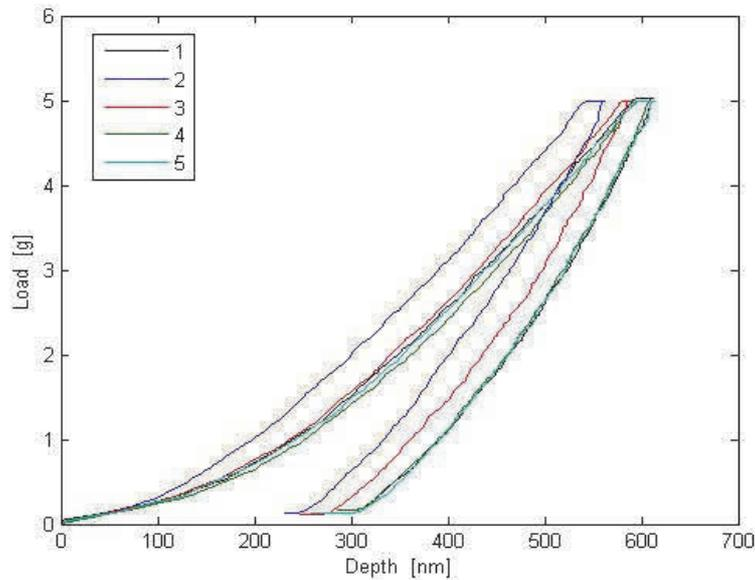
**Figure 2** Indentation curves from measurement by maximal load 5 g
