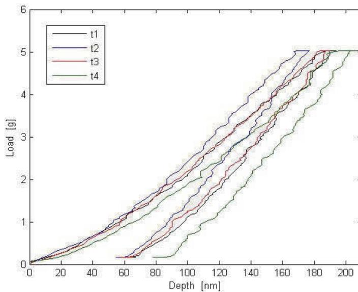
**Figure 5** Indentation curves with maximal load 2 g
