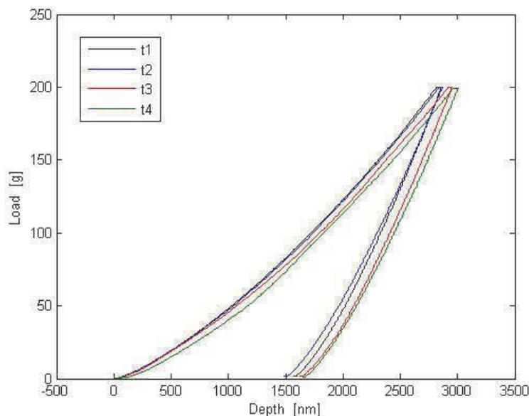
**Figure 3** Indentation curves with maximal load 200 g
