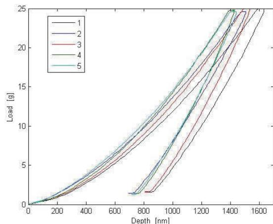
**Figure 1** Indentation curves from measurement by maximal load 25 g
