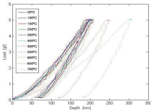
**Figure 7** Comparison of indentation curves with maximal load 5g on sample after temperature loading from 20 C to 750 C
