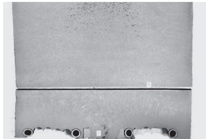
Figure 3 Macrostructure in the axis of uncooled and cooled ingot, detail of the bottom part of ingots
