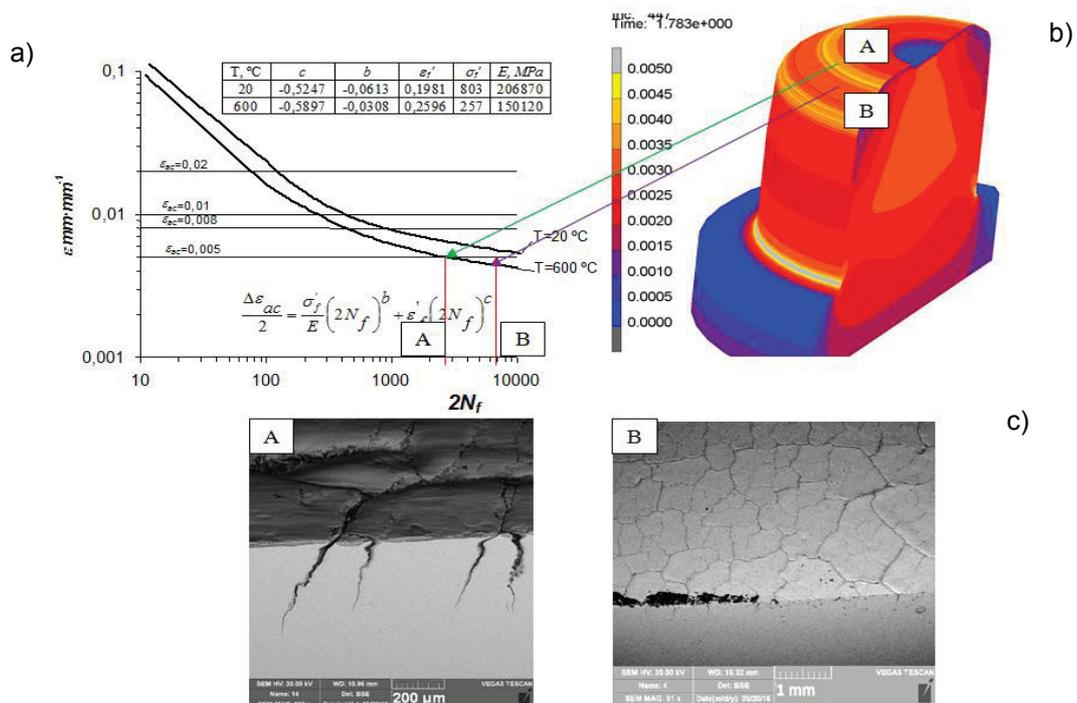
**Figure 6** The view of: a) fatigue charts from a deformation perspective, b) results of FEM simulation - distributions of total deformation, c) photographs of microstructure in selected areas of a tool after 4000 forgings: A - 0.005 deformation - visible network of thermomechanical fatigue cracks along with deep cracks, B - 0.003 deformation - visible mild crack network of thermal origin
