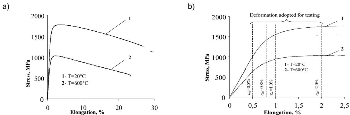
**Figure 4** Results of static tests: a) tensile charts, b) initial area of the chart to selection of strain amplitude
