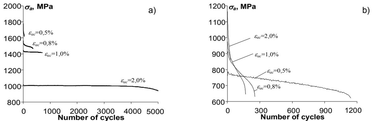
**Figure 5** Changes of stress  $\varepsilon_a$  as a function of the number of loading cycles: a)  $T = 20\text{ }^\circ\text{C}$ , b)  $T = 600\text{ }^\circ\text{C}$
