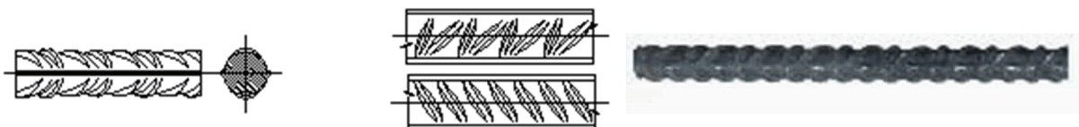
Figure 1 The geometry of the ribbed bars made of steel BSt500S [13]
