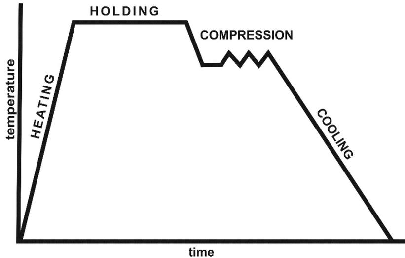
**Figure 2** Schematic representation of the compression tests performed on Bähr MDS 830
