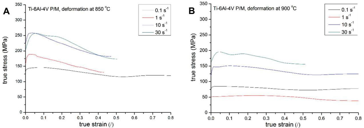
**Figure 4** Stress-strain curves obtained in compression tests of P/M Ti-6Al-4V alloy at the temperatures of 850 °C (A) and 900 °C (B)
