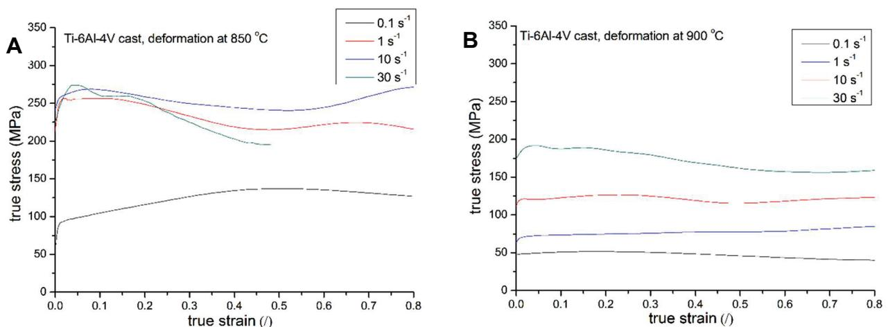
**Figure 3** Stress-strain curves obtained in compression tests of cast Ti-6Al-4V alloy at the temperatures of 850 °C (A) and 900 °C (B)
