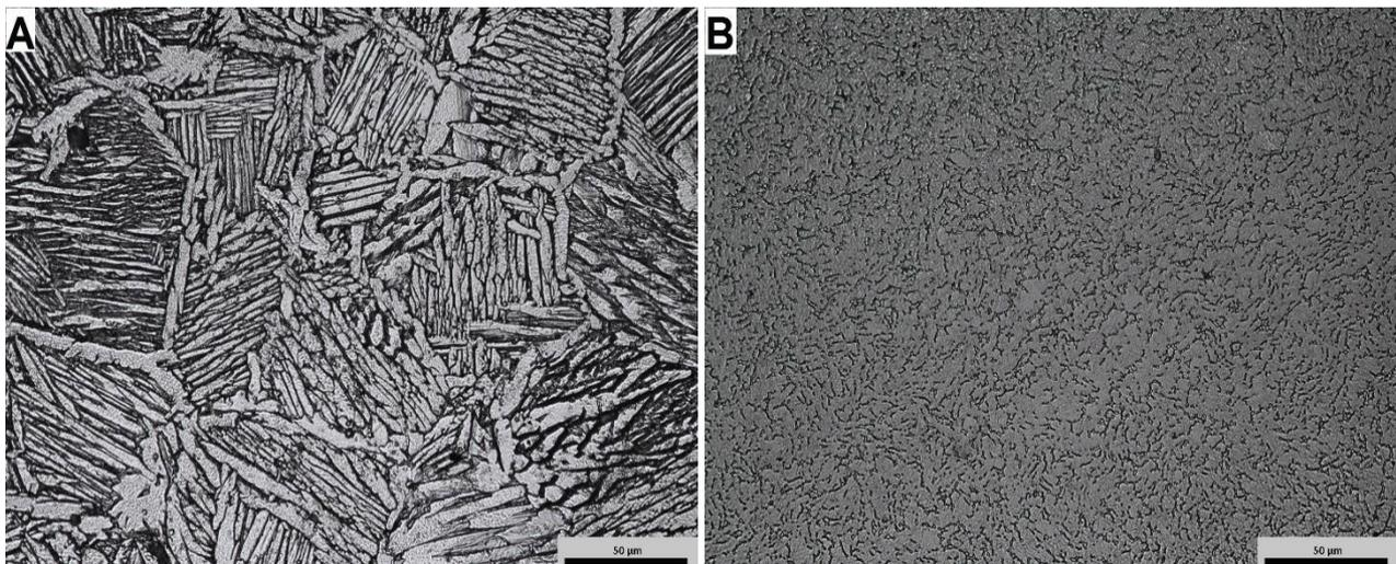
**Figure 1** Microstructure of as-received P/M (A) and cast (B) Ti-6Al-4V alloy
