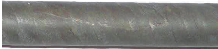
Figure 6 Shape of the 7075 aluminum alloy bars obtained in three-high skew rolling mill
