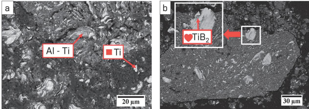
**Figure 3** A cross-sectional SEM microstructures of powder mixture milled for (a) 2 and (b) 6 hours
