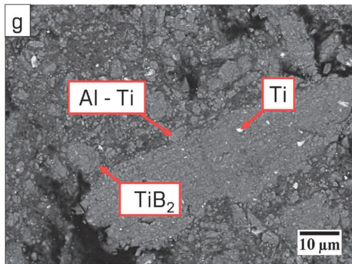
**Figure 6** A cross - sectional SEM micrographs of powder mixture milled for (g) 40 hours
