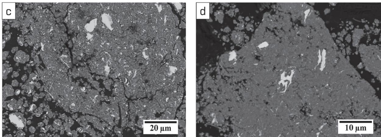
**Figure 4** The cross-sectional SEM microstructures of powder mixture milled for (c) 10 and (d) 20 hours
