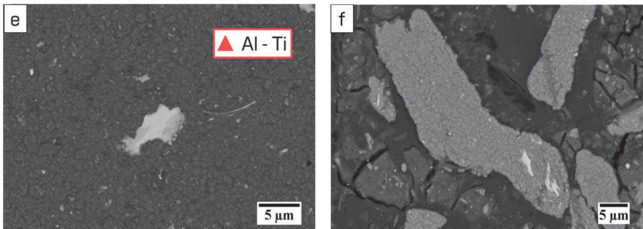
**Figure 5** The SEM microstructures of powder mixture milled for (e) 25 and (f) 30 hours
