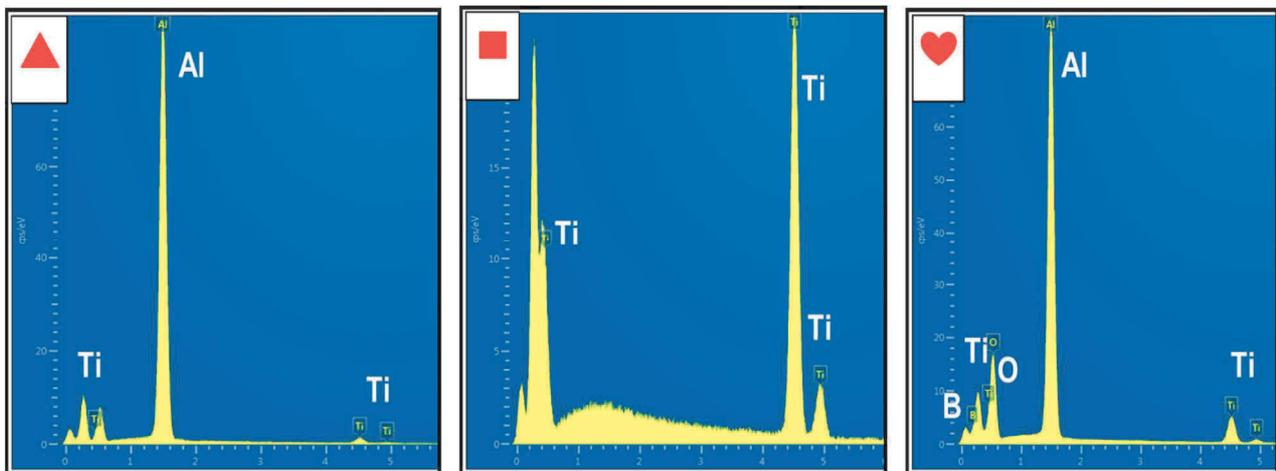
**Figure 7** EDS analysis of selected areas of Al - Ti; titanium and TiB<sub>2</sub>
