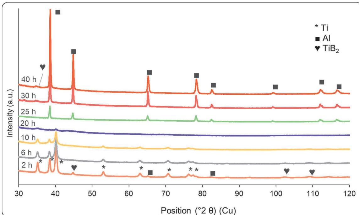
**Figure 1** The XRD patterns of sample milled for 2, 6, 10, 20, 25, 30 and 40 hours
