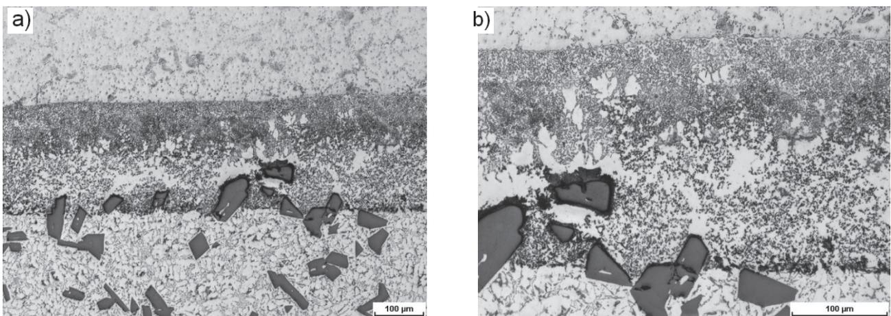
**Figure 2** Microstructures of the bonding zone between the AZ91 and the unrefined AlSi17: (a) lower magnification, (b) higher magnification
