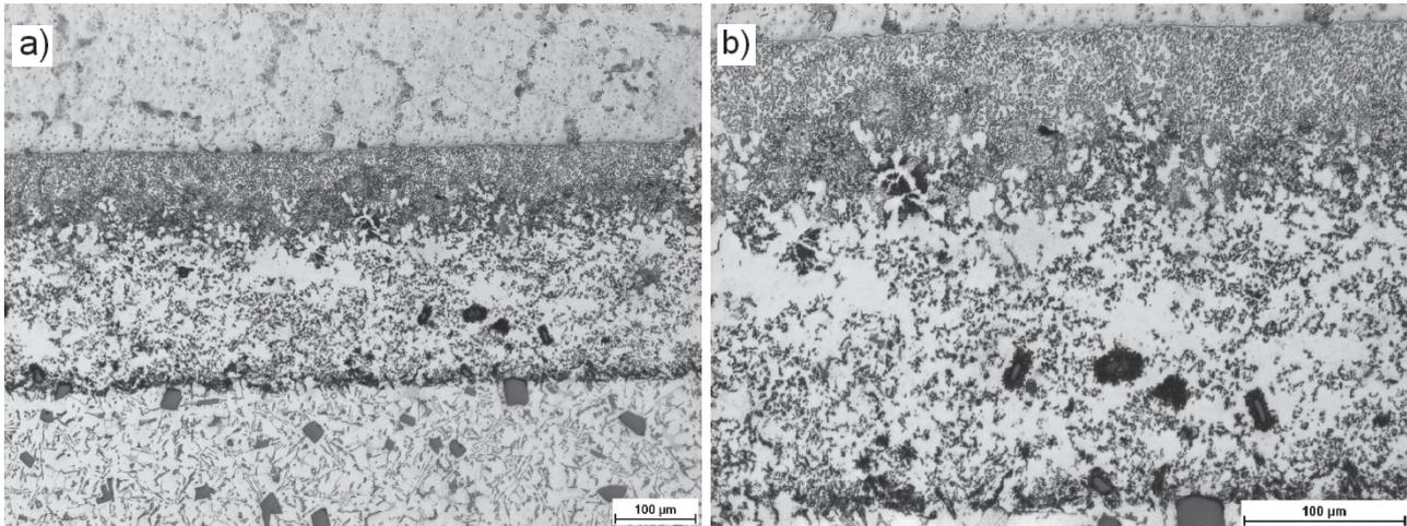
**Figure 4** Microstructure of the bonding zone formed between the AZ91 and the insert cut from rapidly solidified AlSi17 alloy, (a) lower magnification, (b) higher magnification
