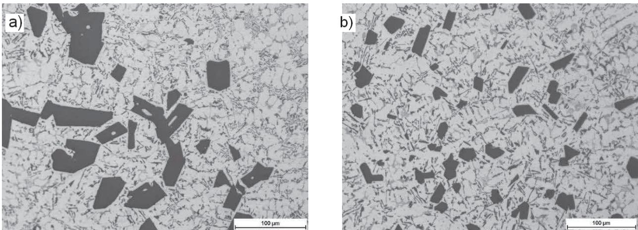
**Figure 1** Microstructures of the AlSi17 inserts: (a) cut from the AlSi17 ingot, (b) cut from the rapidly solidified AlSi17 alloy
