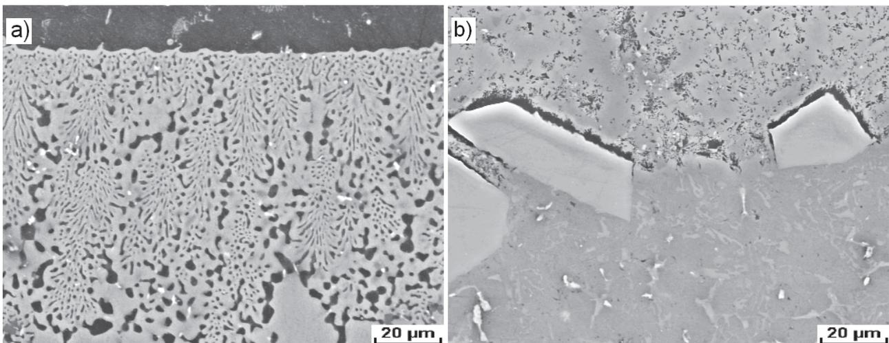
**Figure 3** Details of the microstructure of the bonding zone between the AZ91 and the unrefined AlSi17 observed by SEM: (a) AZ91 side, (b) AlSi17 side
