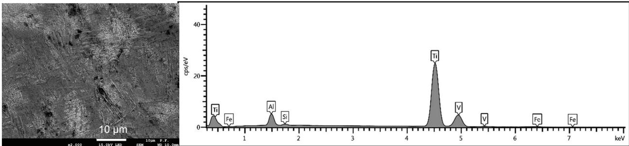
**Figure 3** The structure of WZ by EBW methods and EDS
