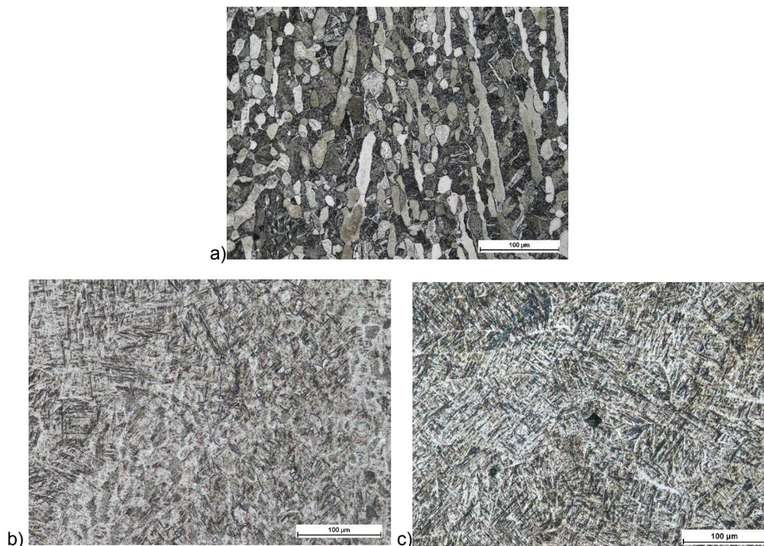
**Figure 2** Microphotography of weld structure a) BMZ; b) HAZ c) WZ
