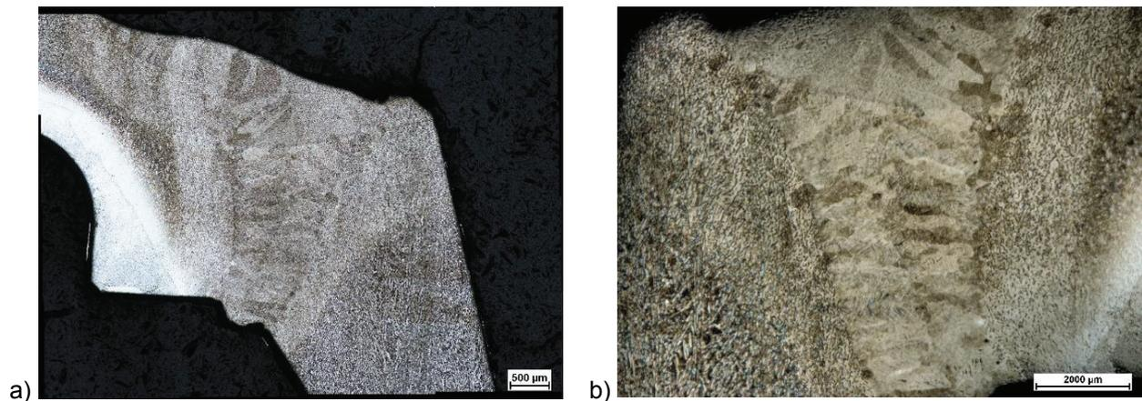
**Figure 1** Macrophotography of weld structure
