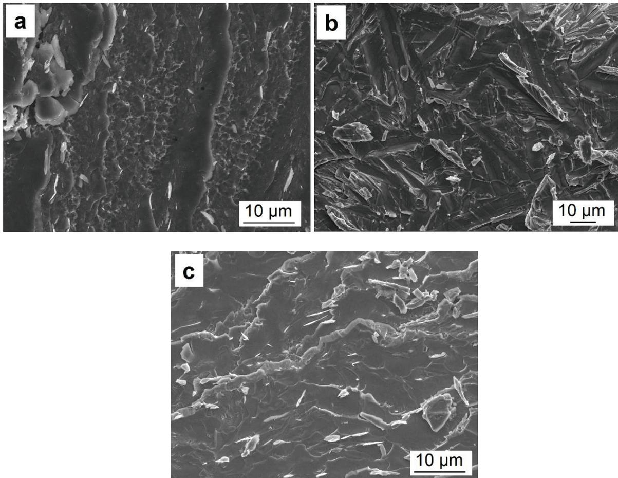
**Figure 2** Fracture surfaces of the brazed joints processed by a) Al, b) Cu and c) Ni foils
