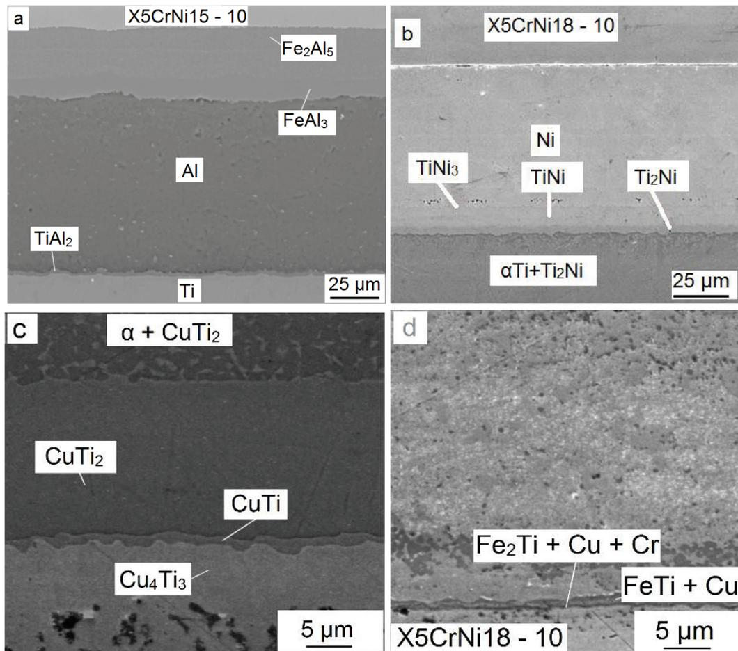
**Figure 1** SEM images of diffusion bonded joint by a) Al, b) Ni, c) Cu (Ti-side), d) Cu (SS-side)
