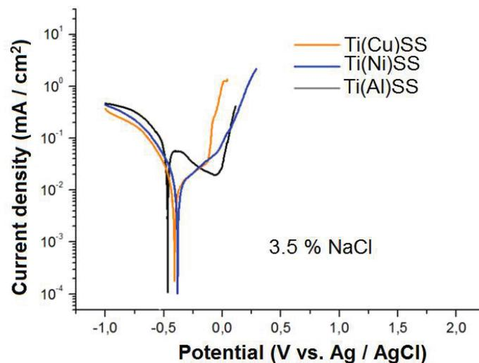
**Figure 3** Polarization curves recorded in 3.5 % NaCl solution for diffusion bonded joints
