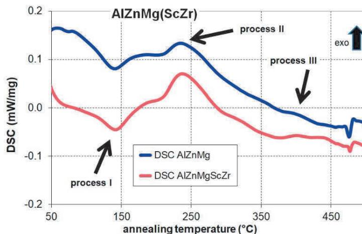
**Figure 2** DSC curves in linear heating rate 20 K/min of the AlZnMg(ScZr) alloys up to 480 °C
