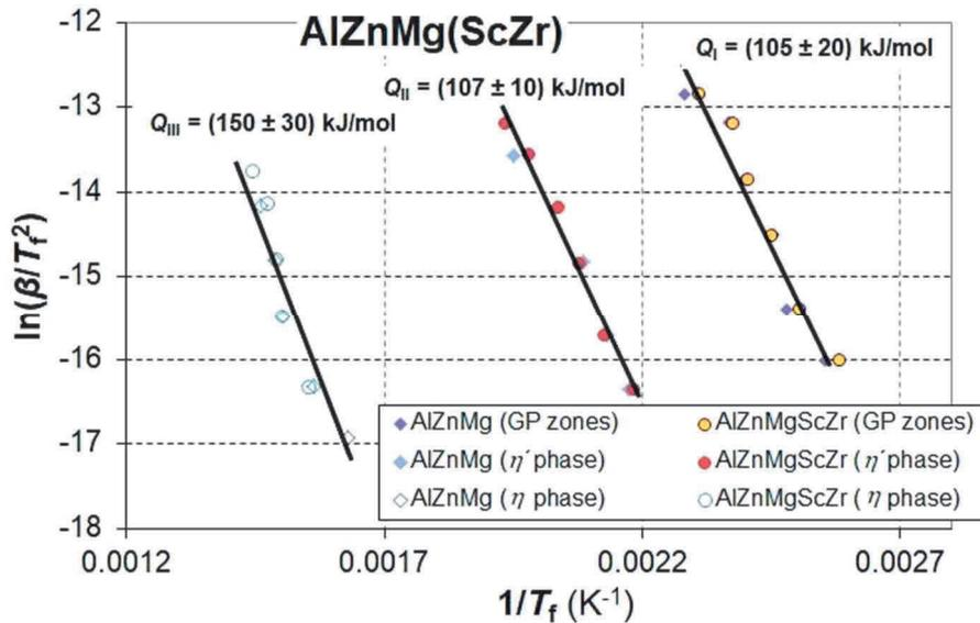
**Figure 4** Kissinger plot in the coordinate system of  $[\ln(\beta/T_f^2); 1/T_f]$  of the heat effects in the AlZnMg(ScZr) alloys,  $\beta$  is the linear heating rate  $[K \cdot s^{-1}]$ ;  $T_f$  is the peak temperature of DSC trace for particular heat effects
