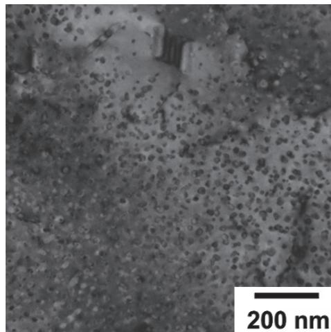
**Figure 3** TEM image of the AlZnMg alloy isochronally annealed up to 220 °C. See particles of the  $\eta'$  phase
