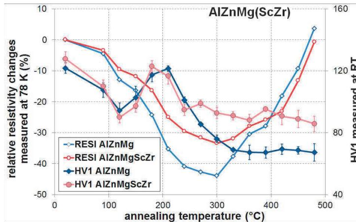
**Figure 1** Isochronal annealing curves of relative resistivity changes (measured at 78 K) and microhardness HV1 changes (measured at RT) with standard deviation
