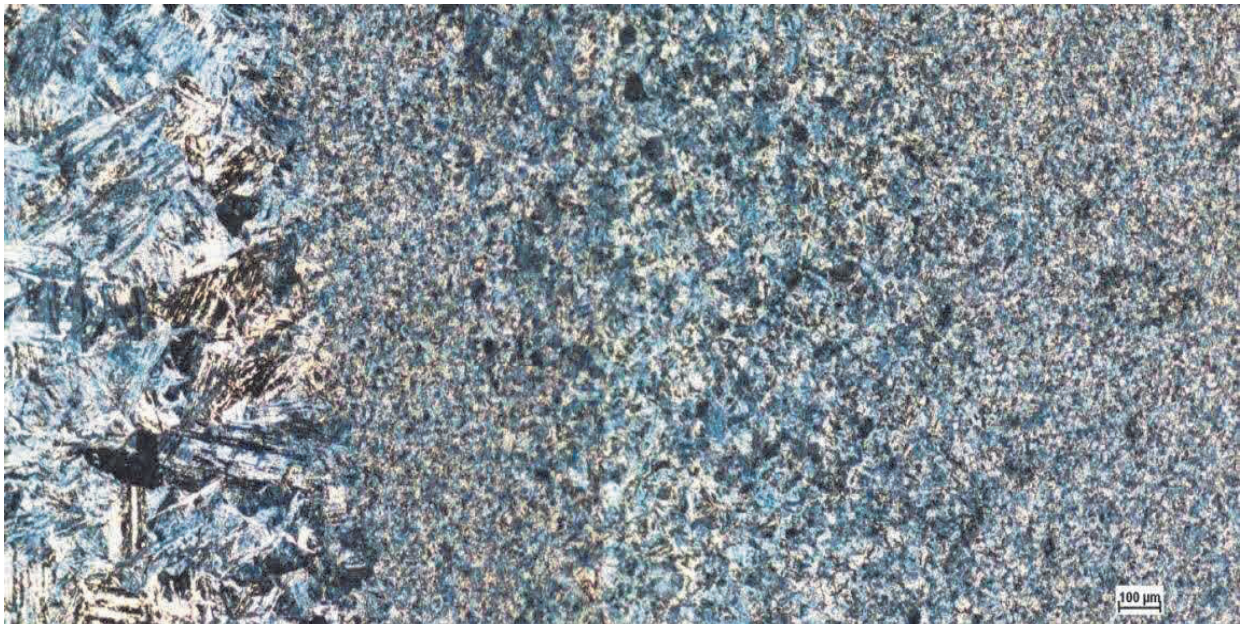
Figure 3 Microphotography of X10CrMoNb9-1 steel with the deposited weld electrode alloy W CrMo2Si by TIG welding
