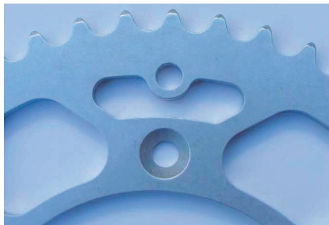
Figure 3 The macrophotography fragment of sprocket wheel after vibratory tumbling
