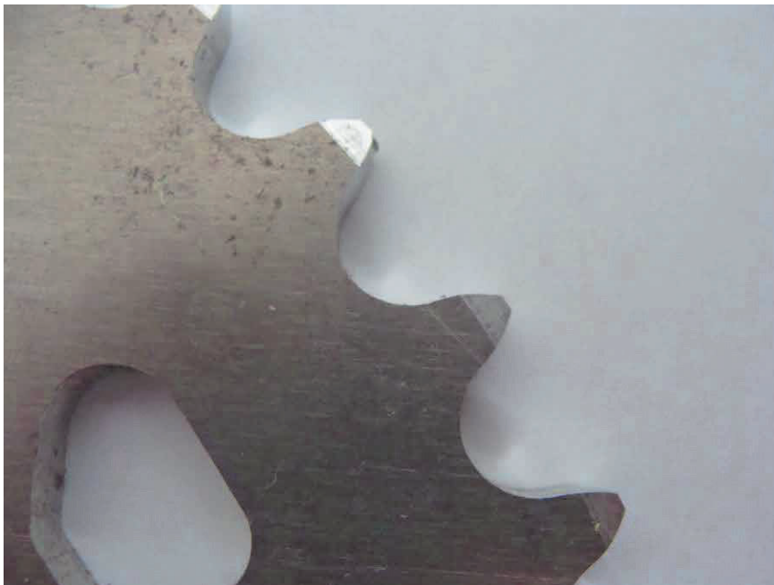
Figure 1 Fragment of sprocket - the sharp edges and discoloration incurred in the sprocket wheel
