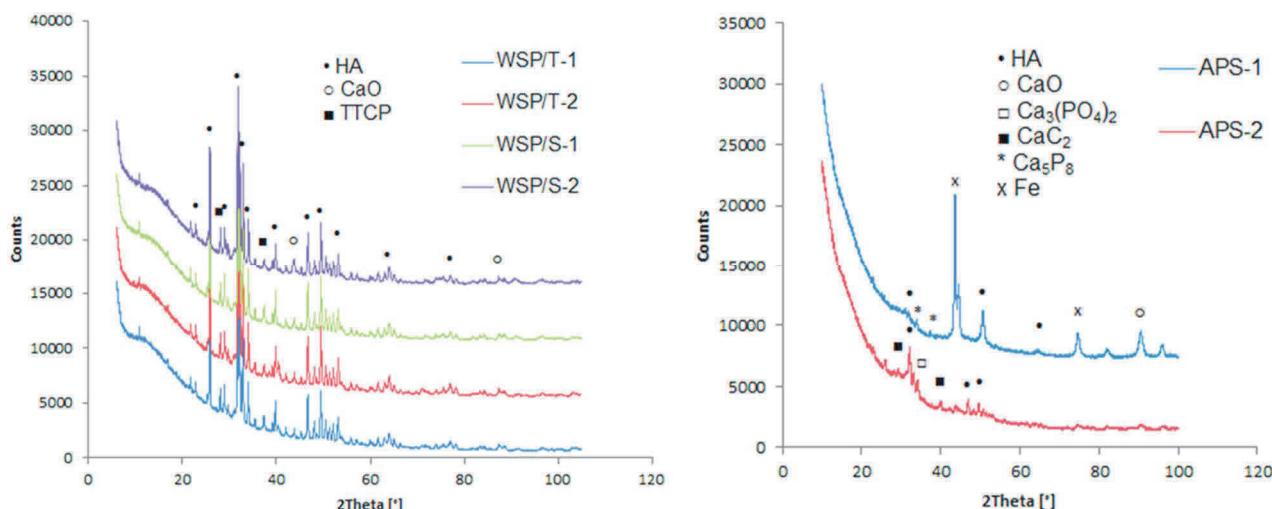
**Figure 2** XRD patterns of the HA layers produced via WSP-H and APS technologies
