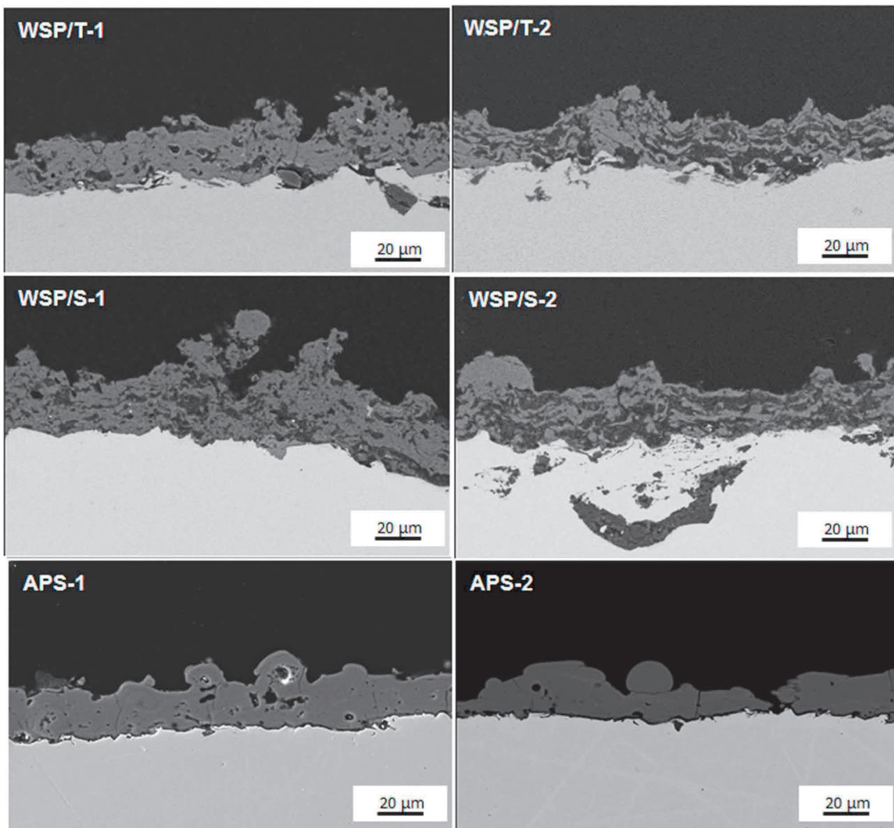
**Figure 1** The structure of HA coatings produced via WSP-H and APS technologies
