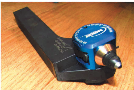
Figure 2 External reaming tool with diamond tip
