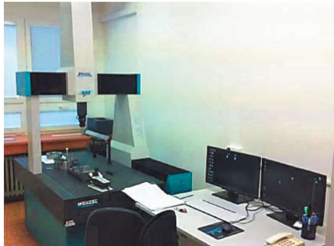
Figure 8 Wenzel LH65 X3M Premium coordinate measuring machine
