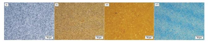
**Figure 1a** Microstructure of the titanium alloy 100% Ti-6Al-4V (bulk alloy): a) before thermal oxidation and after thermal oxidation at temperatures: a') 400°C, a'') 500°C, a''') 600°C
