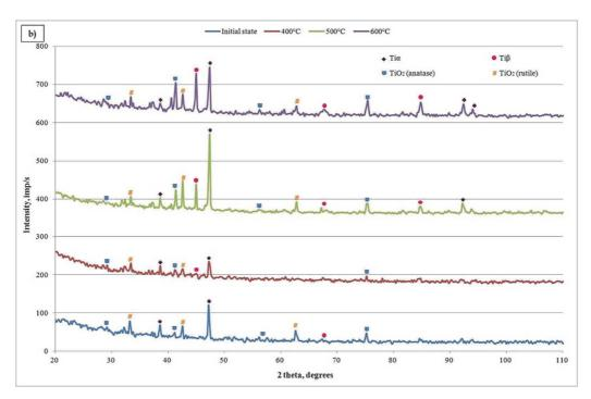
**Figure 4** Diffractograms of the titanium alloy after thermal oxidation at appropriate temperatures: a) 100% Ti-6Al-4V (bulk alloy), b) 100% Ti-6Al-4V (porous sinters)
