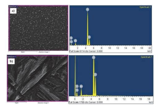
Figure 3 Analysis of chemical composition (Spectrum 1): a) 100% Ti-6Al-4V (bulk alloy) after thermal oxidation at temperature 400°C, b) 100% Ti-6Al-4V (porous sinters) after thermal oxidation at temperature 500°C
