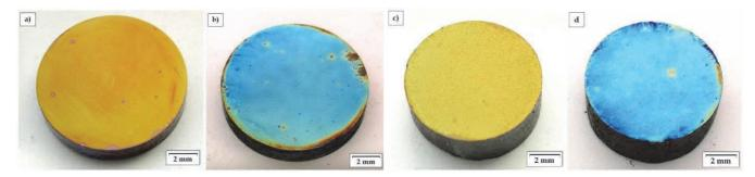
**Figure 2** Macroscopic images of the titanium alloys after thermal oxidation at appropriate temperatures: a) 100% Ti-6Al-4V (bulk alloy) at 500°C, b) 100% Ti-6Al-4V (bulk alloy) at 600°C, c) 100% Ti-6Al-4V (porous sinters) at 500°C, d) 100% Ti-6Al-4V (porous sinters) at 600°C
