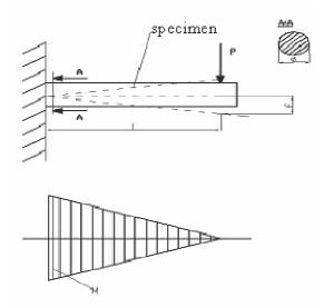
Figure 1 A scheme of the measured system and a diagram of bending moments: P - load, f - deflection
