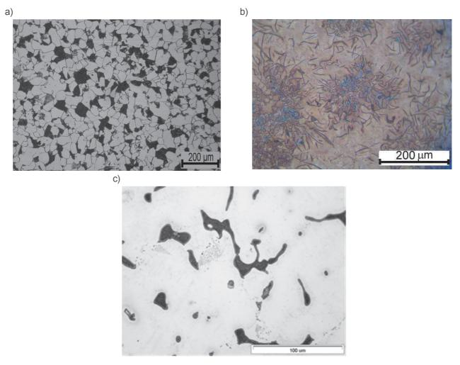
Figure 2 The structures of alloys in this study: a) steel with ferritic-pearlitic structure, b) a flake cast iron, c) an aluminum magnesium alloy
