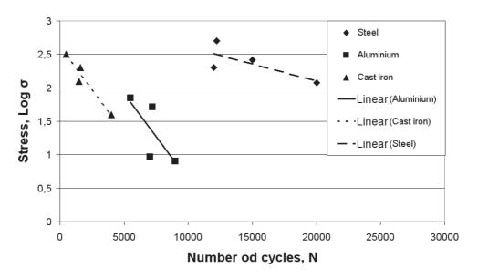
Figure 4 A diagram of the fatigue strength as a function of the number of cycles
