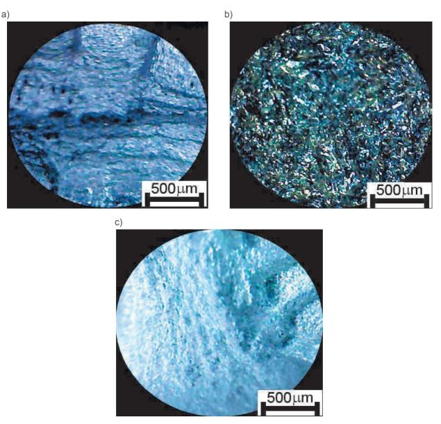
Figure 5 The surface of fatigue fracture: a) a sample from steel, b) samples of cast iron, c) samples of aluminium alloy
