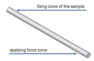
Figure 3 Form of material sample taken from the swingarm
