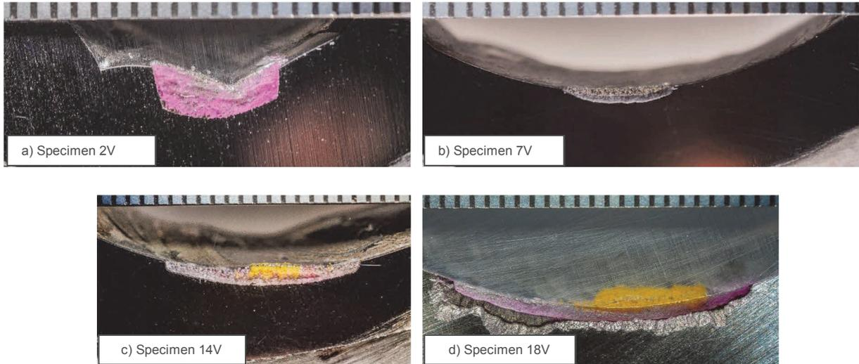
**Figure 3** Appearance of the inner surface of tubular bodies with detected defects (cross-section of defects)
