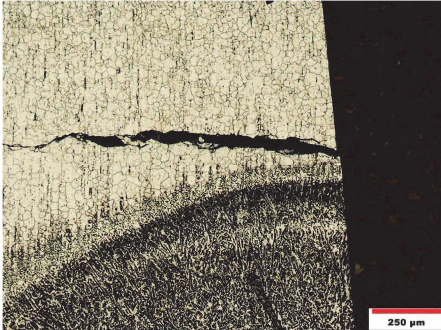
**Figure 8** Crack in the HAZ area (specimen 18V)
