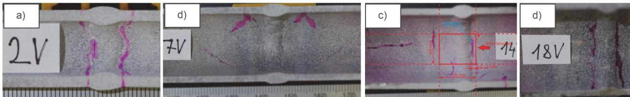
**Figure 2** Appearance of inner surface of tubular bodies with detected defects
