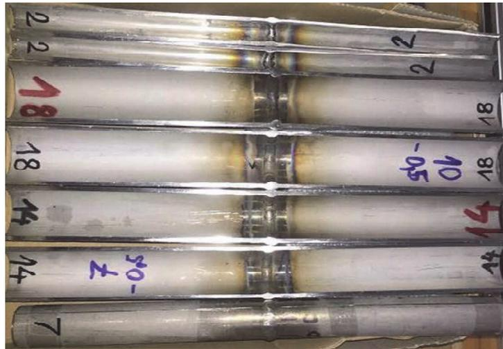
**Figure 1** Tubular bodies after longitudinal cutting
