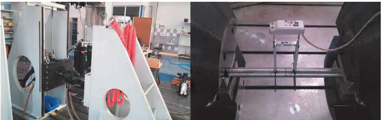
Figure 2 Electro-hydraulic test stand and mounted bar specimen
