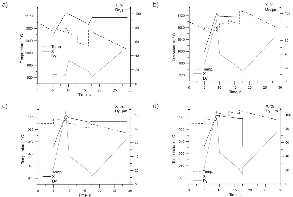
**Figure 4** Results of calculation of dynamic recrystallized austenite grain size and recrystallized fraction for various locations: a), b) surface, c), d) core of the head (point A) and the shank (point B), respectively
