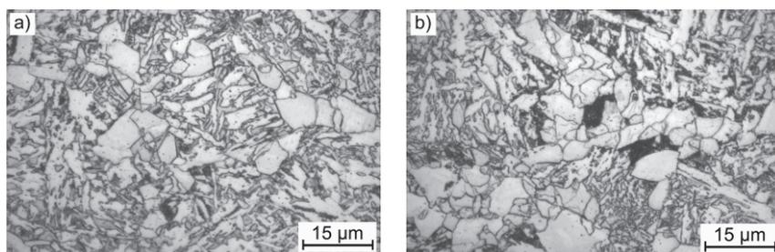
**Figure 5** Reference microstructure of the analyzed forged part in section A: a) surface, b) core
