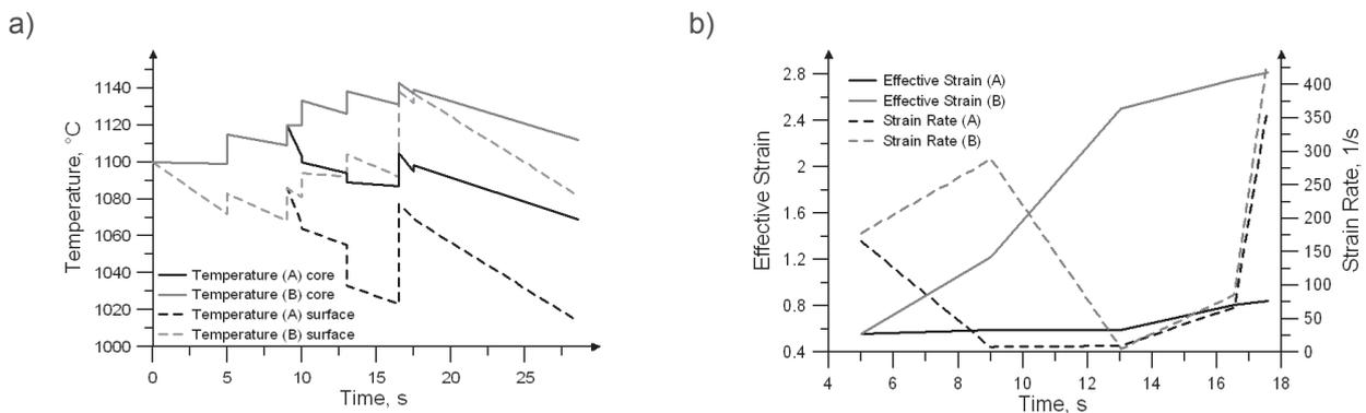
**Figure 3** Numerically established history of: a) temperature, b) effective strain and effective strain rate
