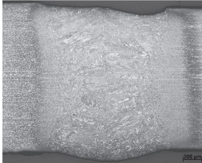
Figure 1 Macrostructure of welded joint of 780C steel with 690T steel
