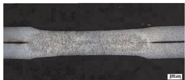
D - Unacceptable electrode indentation
