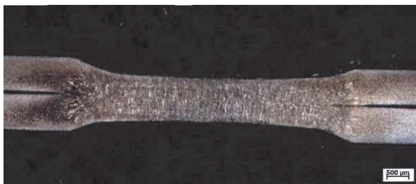
C - Size of weld acceptable, traces of Cu
