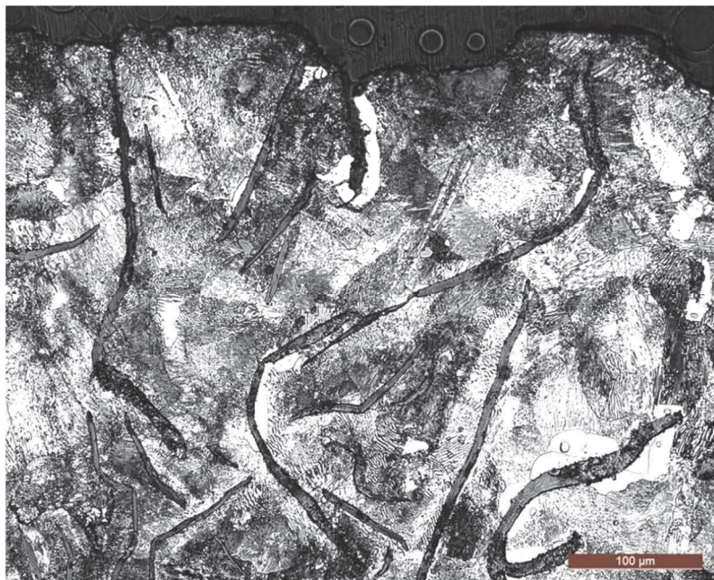
Figure 7 Microstructure of the cavitated sample cross section cavity for 165 min. Etching, NITAL 3%
