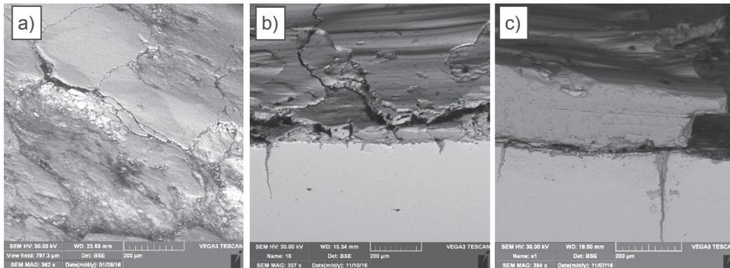
**Figure 5** View of the oxide layer in area 3 on a tool nitrided a) traditionally, b) by ZeroFlow variant no. 1 ( $\epsilon$ ), c) by ZeroFlow variant no. 2 ( $\gamma'$ )
