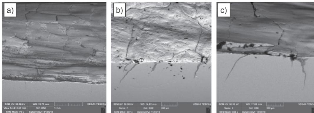
**Figure 4** SEM view of the surface in area no. 1 on a tool nitrided a) traditionally, b) by ZeroFlow variant no. 1 ( $\epsilon$ ), c) by ZeroFlow variant no. 2 ( $\gamma'$ )
