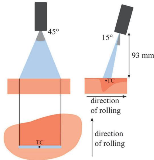
**Figure 1** Diagram of the nozzle configuration
