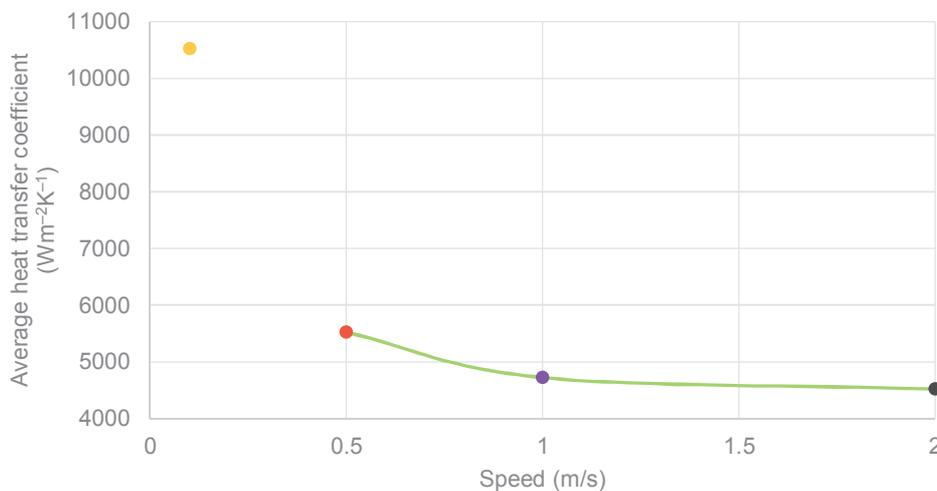
**Figure 7** Average heat transfer coefficient with respect to the speed of the carriage
