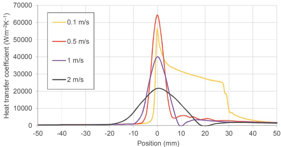
**Figure 6** Heat transfer coefficient with respect to the position of the carriage and its speed
