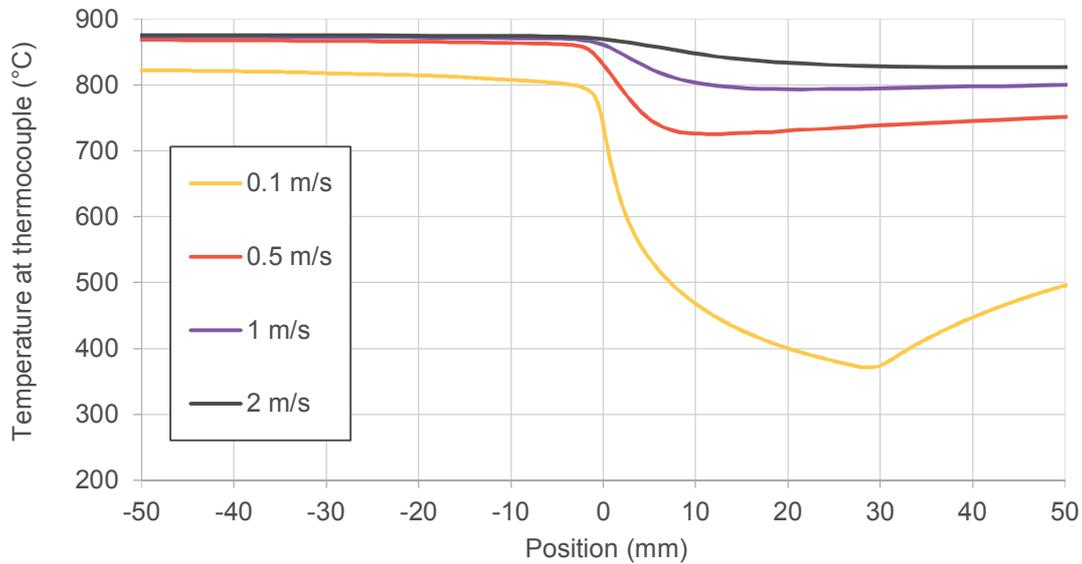
**Figure 4** The temperature of the thermocouple with respect to the position of the carriage and its speed
