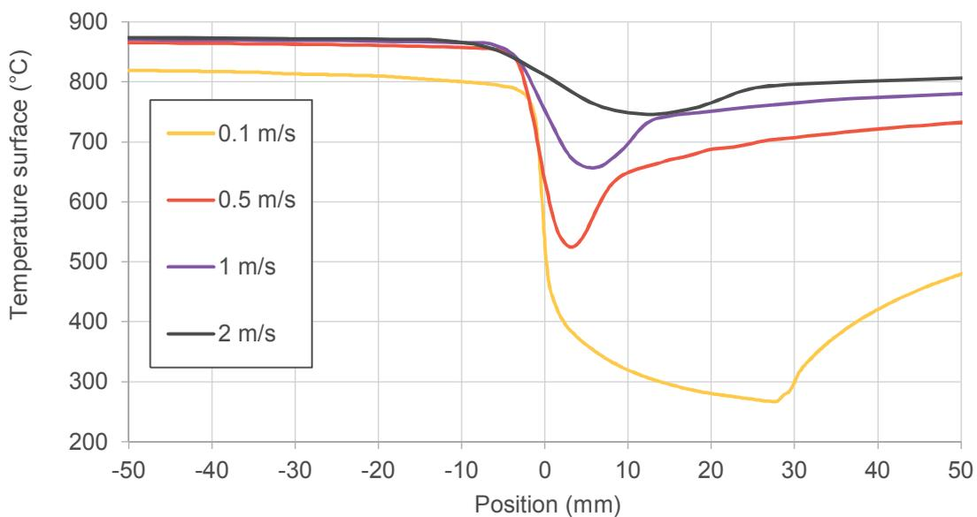
**Figure 5** The temperature of the surface with respect to the position of the carriage and its speed
