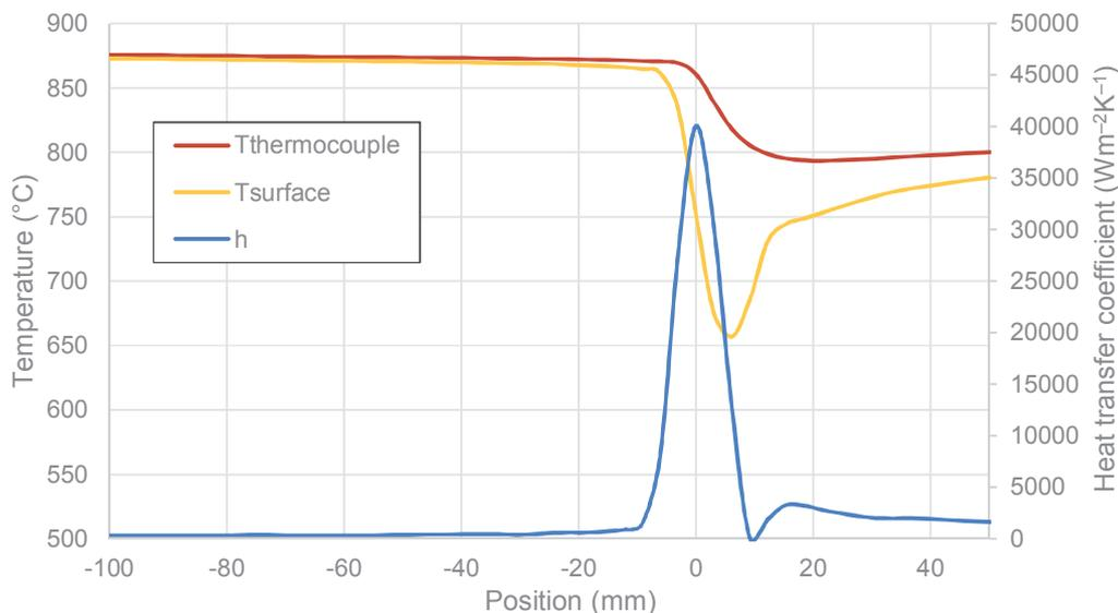
**Figure 3** Measured thermocouple temperature with respect to the position of the carriage. The temperature on the surface and heat transfer coefficient  $h$  was computed by the inverse task algorithm.
