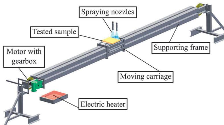
**Figure 2** Diagram of the laboratory bench
