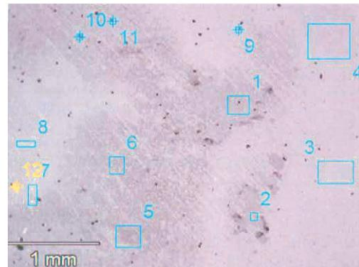
**Figure 7** View of the surface of the drawpiece with marked areas where the SEM EDS analysis was carried out
