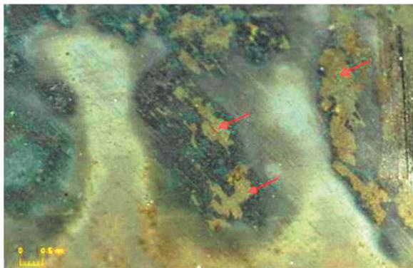
**Figure 6** Stains on the drawpiece surface
