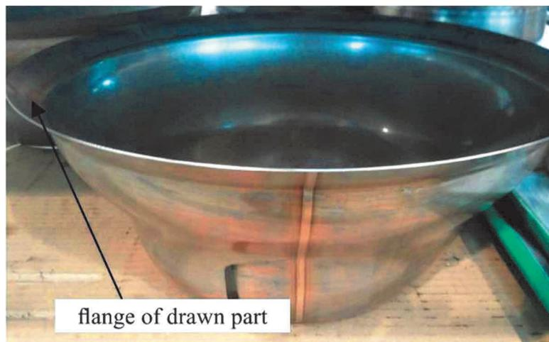
**Figure 4** The shape of the drawpiece after the first forming stage
