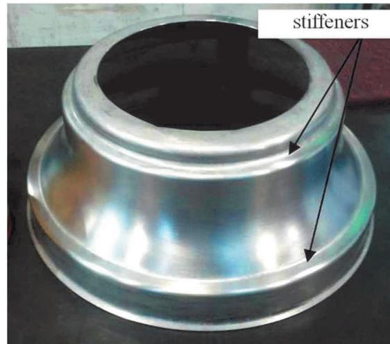
**Figure 3** The fan engine bearing housing element
