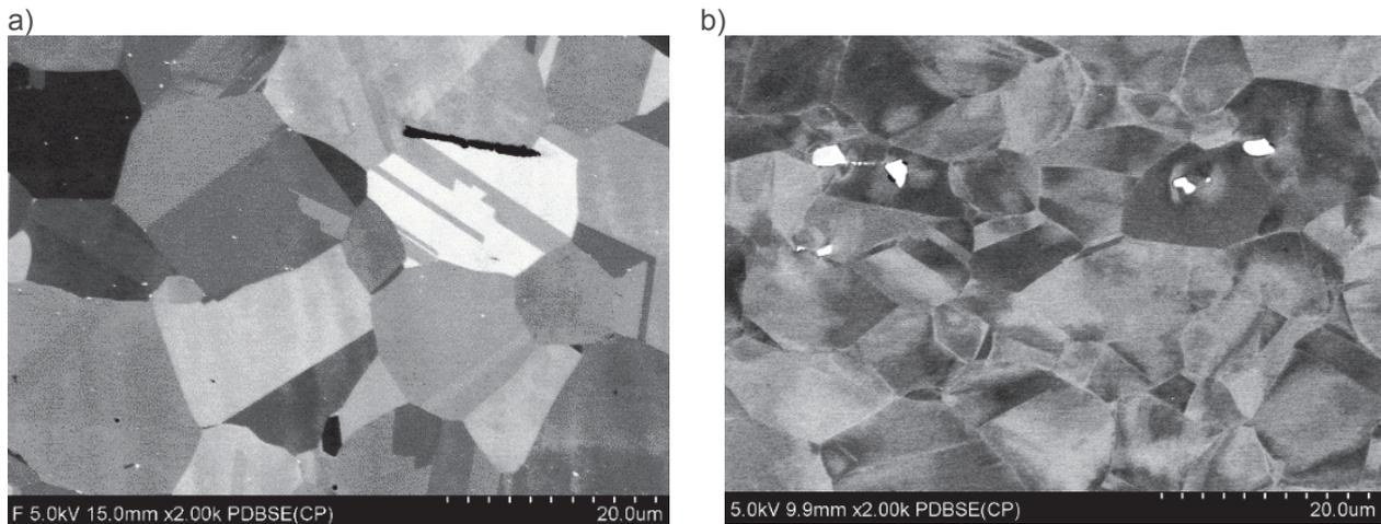
**Figure 3** Pictures from SEM, Inconel 718 in delivery conditions (a) and after plastic deformation in high temperature (b)
