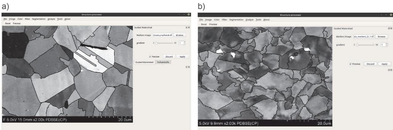
**Figure 6** Grain boundaries determined by the Watershed method
