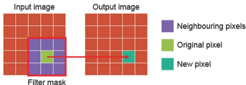
**Figure 2** Image filtering scheme
