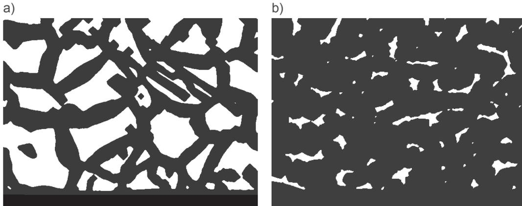
**Figure 5** Marker grid generated for Inconel 718 in delivery conditions (a) for Inconel 718 after plastic deformation (b)
