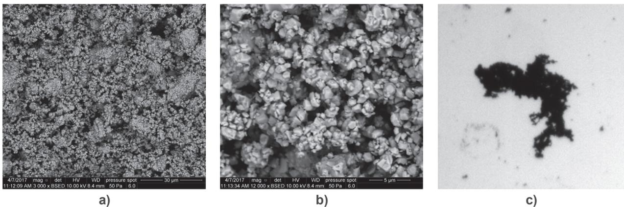
**Figure 5** SEM (a, b) and optical (c) microscopy photos - single particles and aggregates
