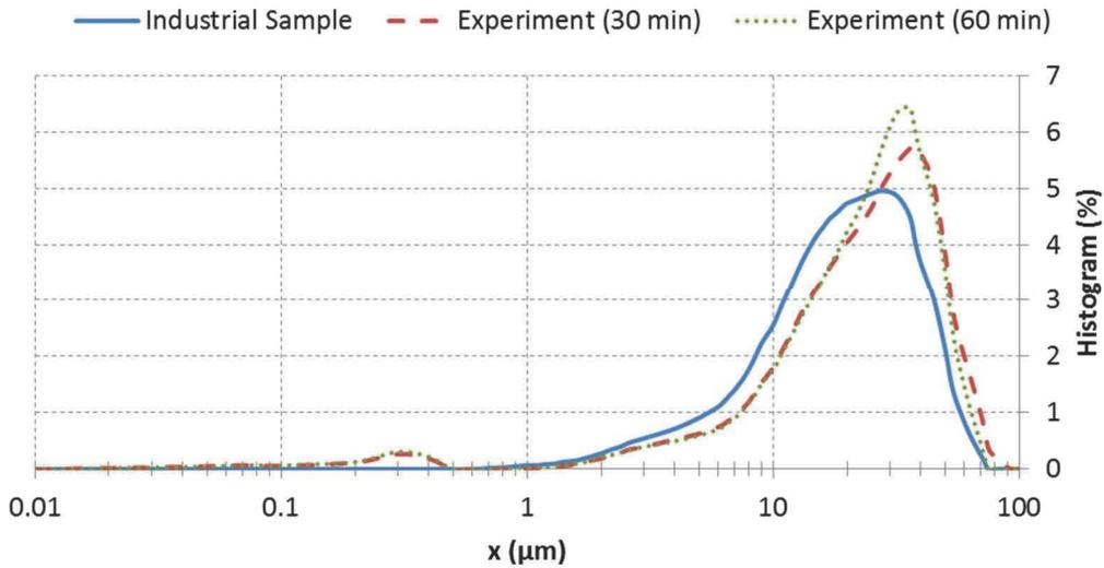
**Figure 4** Particle size distribution of industrial and laboratory samples
