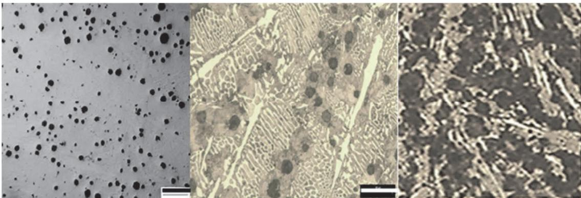
**Figure 5** Nodular iron with 2.49 %Cr (scale 100 µm)
