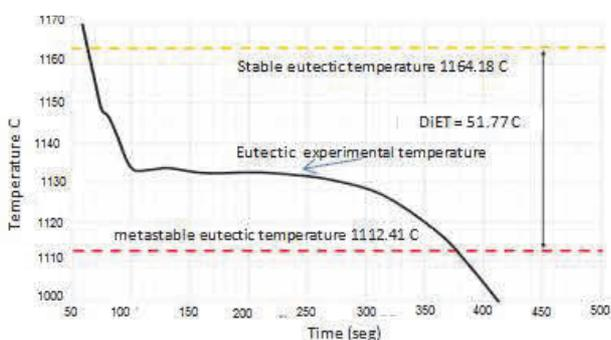
**Figure 6** Cooling curve for iron without chromium
