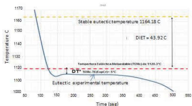
**Figure 7** Cooling curve for iron with 1.35 %Cr
