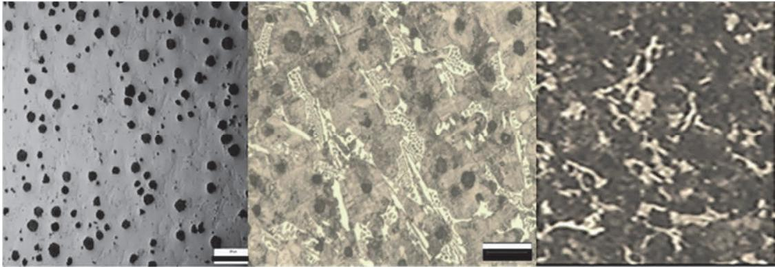
**Figure 3** Nodular iron with 1.35 %Cr (scale 100 µm)
