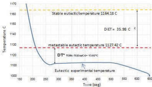
**Figure 8** Cooling curve for iron with 1.95 %Cr
