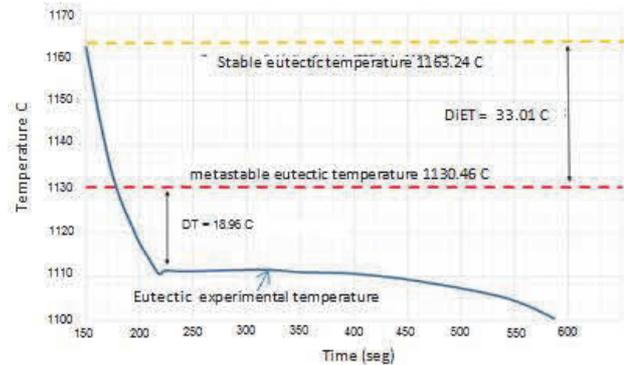
**Figure 9** Cooling curve for iron with 2.49 %Cr
