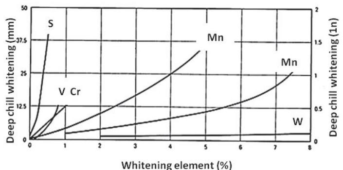
**Figure 1** Whitening power for alloying elements
