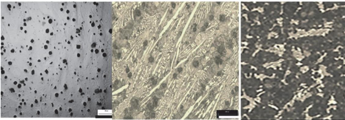
**Figure 4** Nodular iron with 1.95 %Cr (scale 100 µm)
