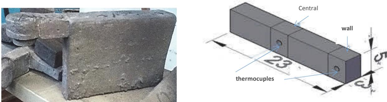
**Figure 2** Y block and segments for metallographic analysis
