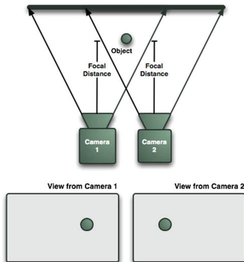
**Figure 2** Illustration of stereoscopy
