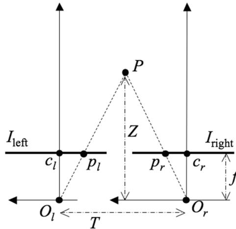
**Figure 3** Schematic of point projection on the image
