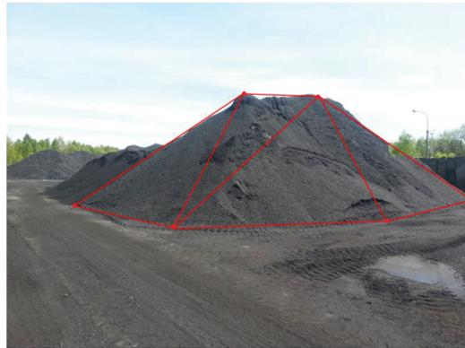
**Figure 5** The low resolution homogeneous yard model
