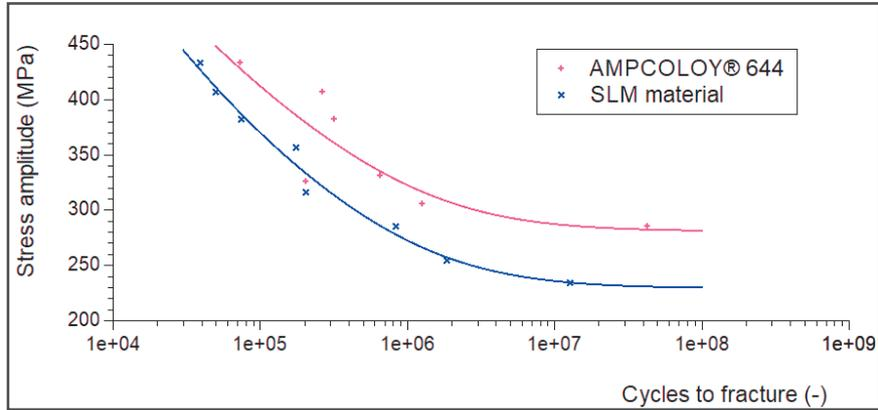
**Figure 4** S-N curves of SLM and AMPCOLOY® 644 materials
