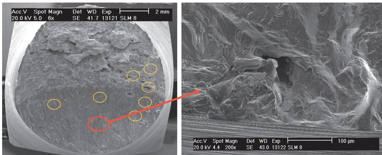
**Figure 6** Fractography of SLM material
