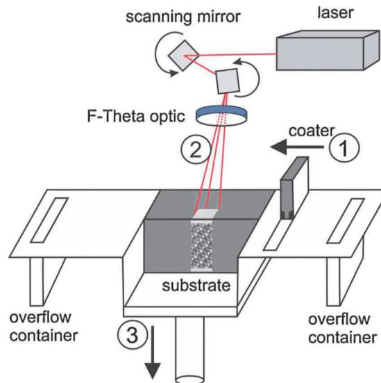
**Figure 1** Selective laser melting principle [1]
