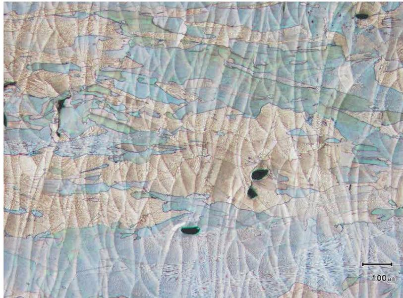
**Figure 2** Microstructure of SLM material
