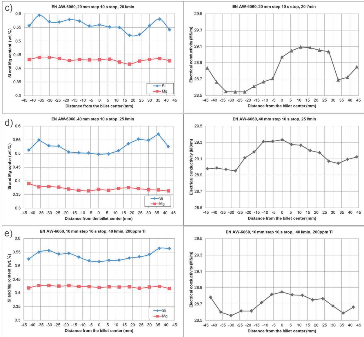
**Figure 3** Deviation of Si and Mg content and changes of electrical conductivity in continuous casting EN AW 6060 aluminum alloy billet 90 mm diameter:
