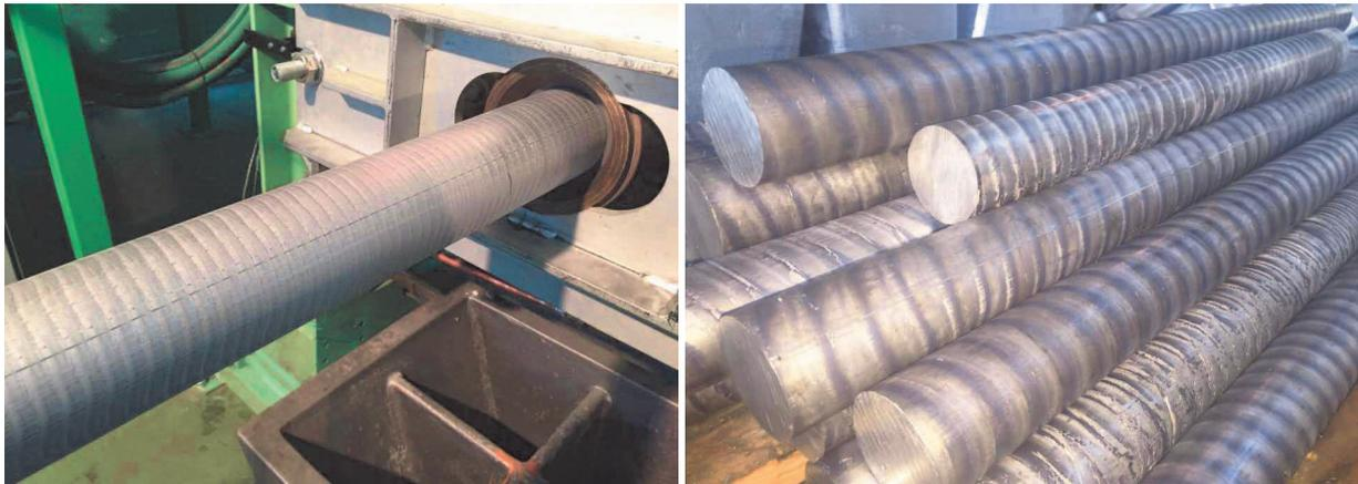
Figure 2b) Industrial continuous casting process and casting rods
