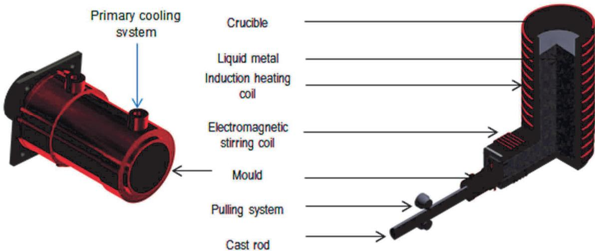
**Figure 2a)** Scheme of continuous casting process
