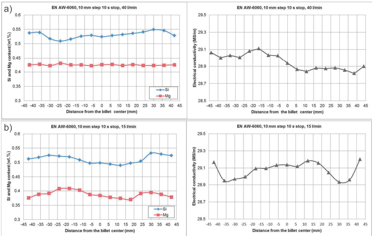
Figure 3 Deviation of Si and Mg content and changes of electrical conductivity in continuous casting EN AW 6060 aluminum alloy billet 90 mm diameter:
