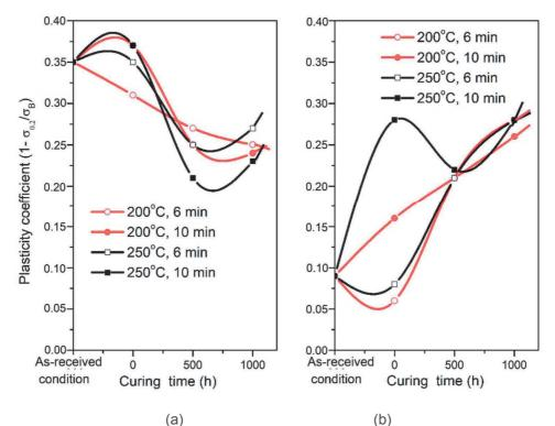
**Figure 4** The effect of operating exposure duration at 150 °C on the plasticity coefficient  $(1 - \sigma_{0.2}/\sigma_{B})$  of 2024 alloy (a) and 1953 (b) after preliminary heating ("0" point) to 200 - 250 °C with the exposure of 6 - 10 min
