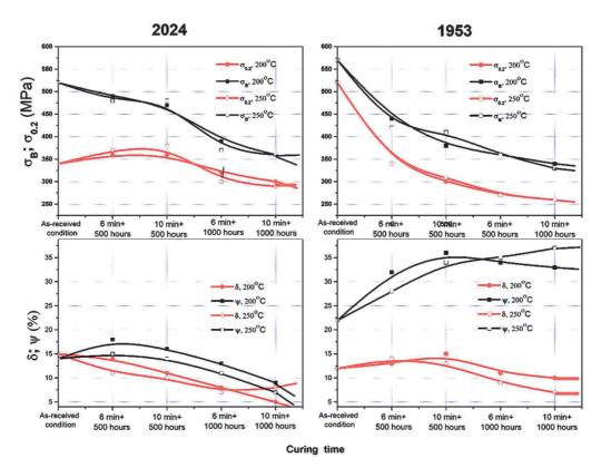
**Figure 5** The influence of exposure duration of 500 or 1000 hours at 150 °C in NaCl + NaOH (pH = 11) on mechanical properties of 2024 and 1953 alloys after preheating (200 or 250 °C, 6 or 10 minutes)
