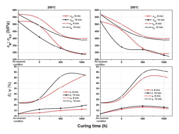
**Figure 3** The effect of operating exposure duration at 150 °C on the mechanical properties of 1953 alloy after preliminary heating ("0" point) to 200 - 250 °C with the exposure of 6 - 10 min
