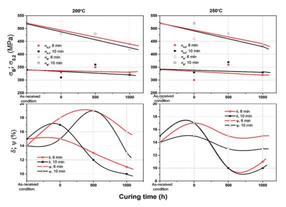
**Figure 2** The effect of operating exposure duration at 150 °C on the mechanical properties of 2024 alloy after preliminary heating ("0" point) to 200 - 250 °C with the exposure of 6-10 min
