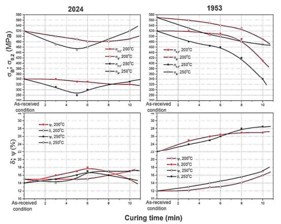
Figure 1 Technological heating duration and temperature effect on the mechanical properties of 2024 and 1953 alloys
