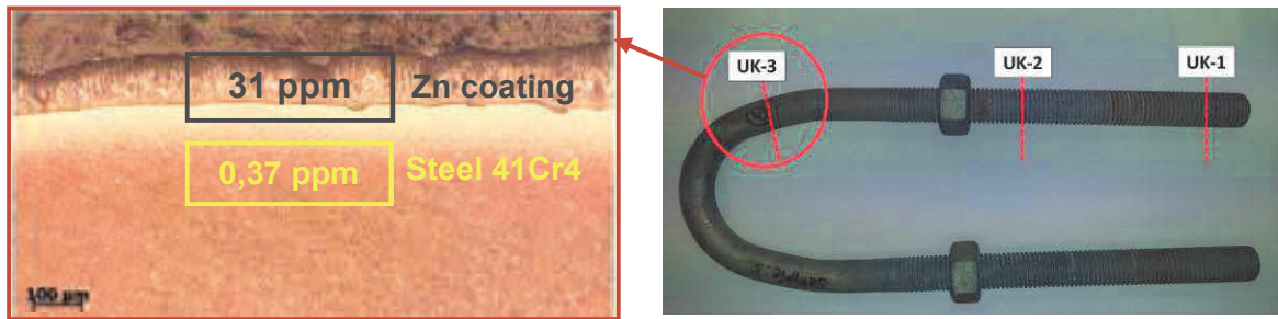
Figure 2 The hydrogen concentration results for samples taken with Zn coating (31 ppm) and without coating (0.37 ppm) [11]
