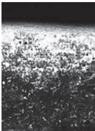
Figure 15 Microstructure after T1, (x100) Nital Attack 2%
