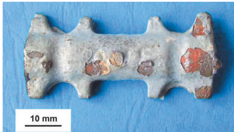
Figure 1 The appearance of overlay with visible corrosion focal points
