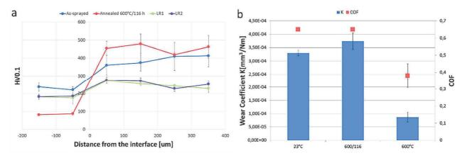
Figure 3 Microhardness depth profile (a) and Coatings Wear coefficient and Coefficient of Friction (b)
