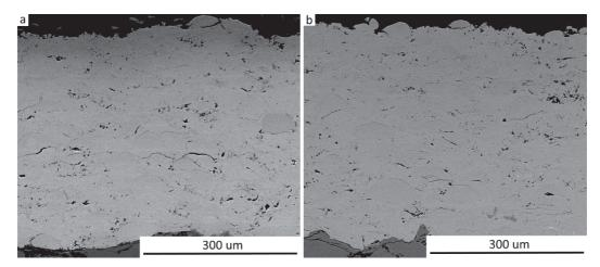
Figure 1 Microstructure of HVOF as-sprayed C-276 coating (a) and furnace annealed coating (b)
