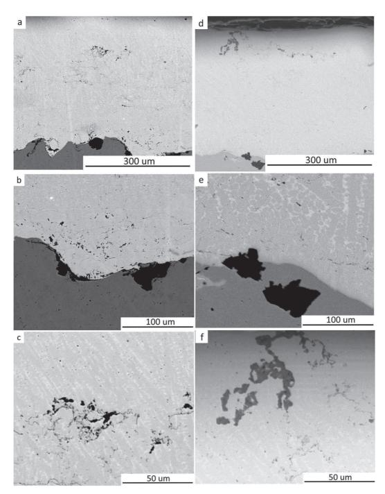
Figure 2 Microstructure of laser remelted coatings by lower (a,b,c) and higher (d,e,f) laser energy specific density
