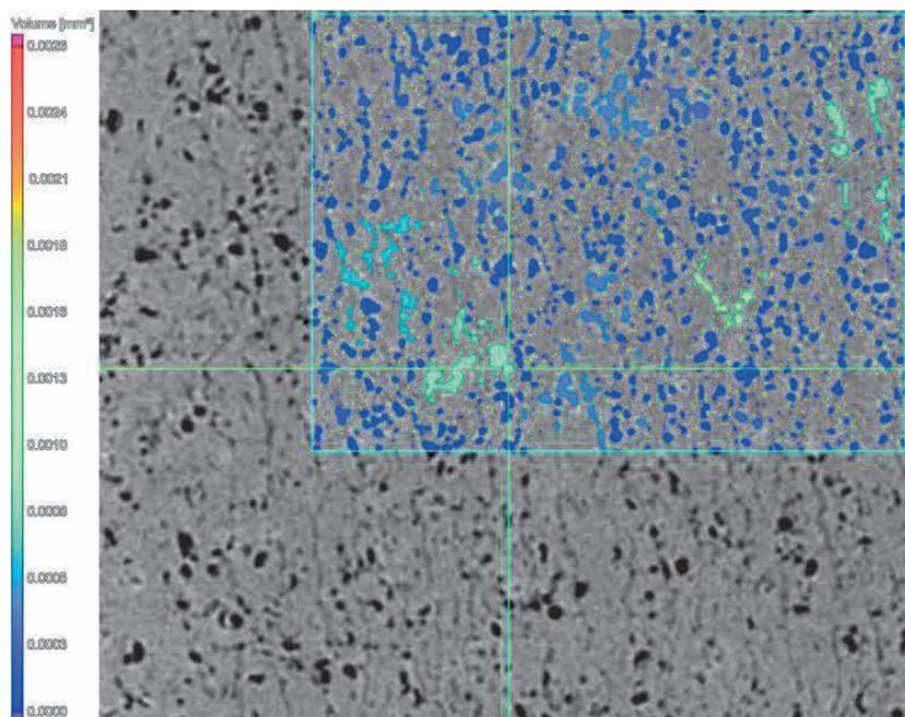
**Figure 4** X-ray tomographic sectional image of plasma sprayed aluminum oxide product
