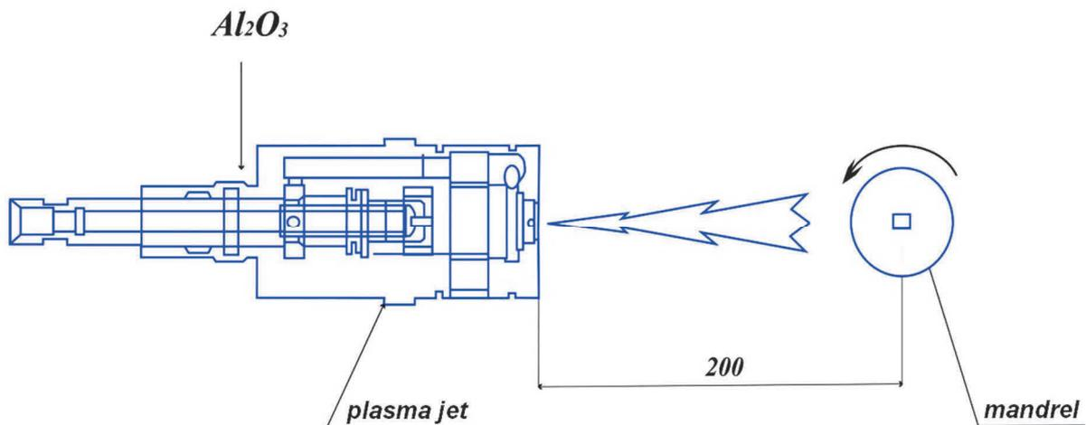
**Figure 2** The scheme of spray deposition
