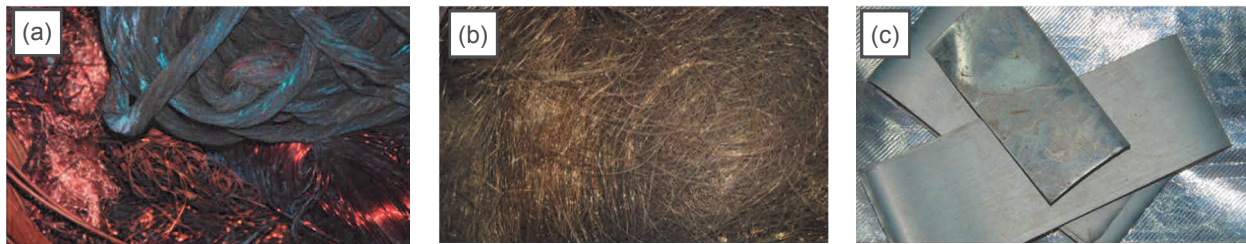
Figure 3 Batch material in scrap used for casting: (a) copper scraps; (b) brass scraps; (c) zinc scraps
