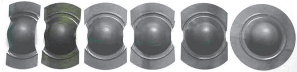
Figure 3 A set of drawpieces to determining forming limit curve
