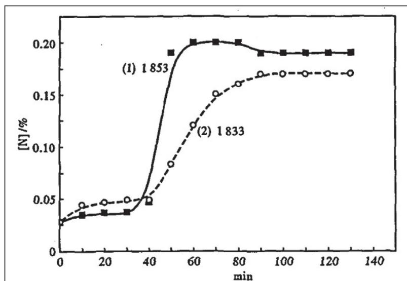
**Figure 3** Nitrogen content in 316L stainless steel melt depending on initial temperature 1,853 K (1,580 °C) and 1,833 K (1,560 °C) and blow time
