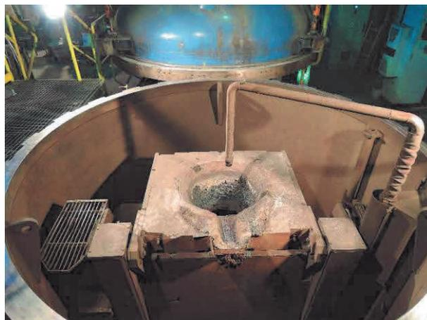
**Figure 5** Vacuum and pressure induction melting furnace with oxygen-nitrogen nozzle, detail
