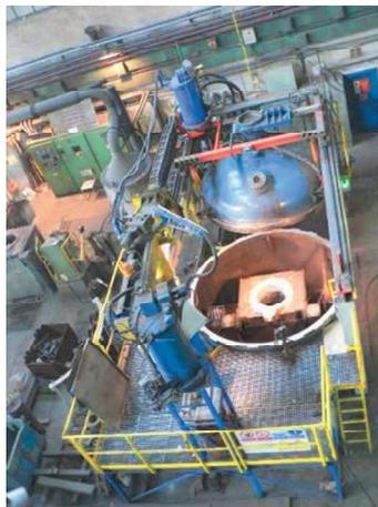
**Figure 4** Vacuum and overpressure induction melting furnace of nominal weight of 1,750 kg
