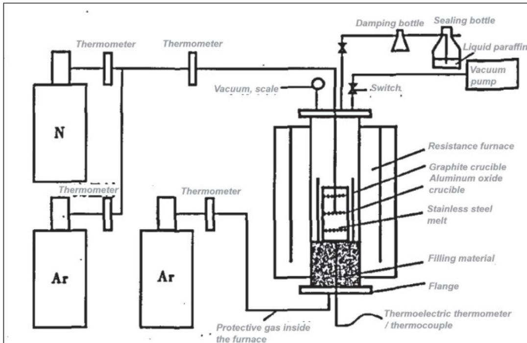
**Figure 2** Experimental device for vacuum nitrogen blowing process
