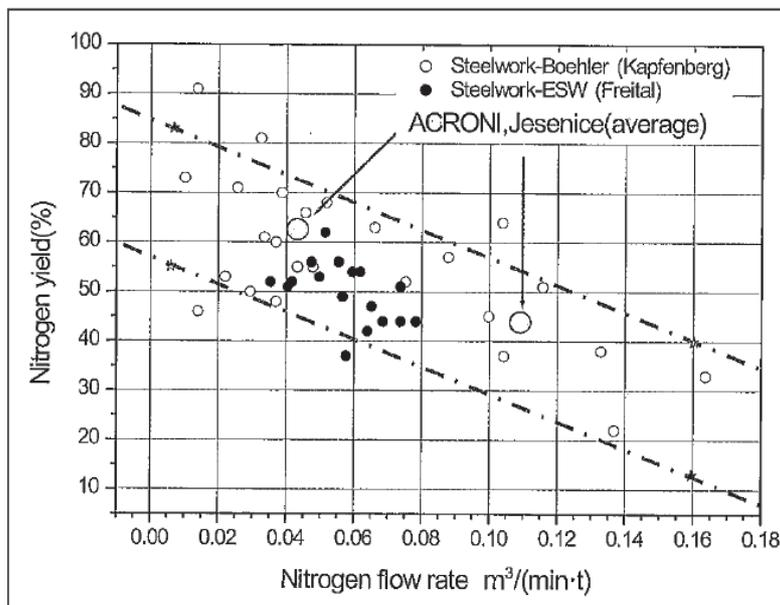
**Figure 1** Efficiency of alloying of nitrogen gas in relation to nitrogen flow in 30 t and 85 t ladle of VOD
