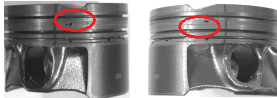
Figure 2 The example of defects created in the casting process [1]
