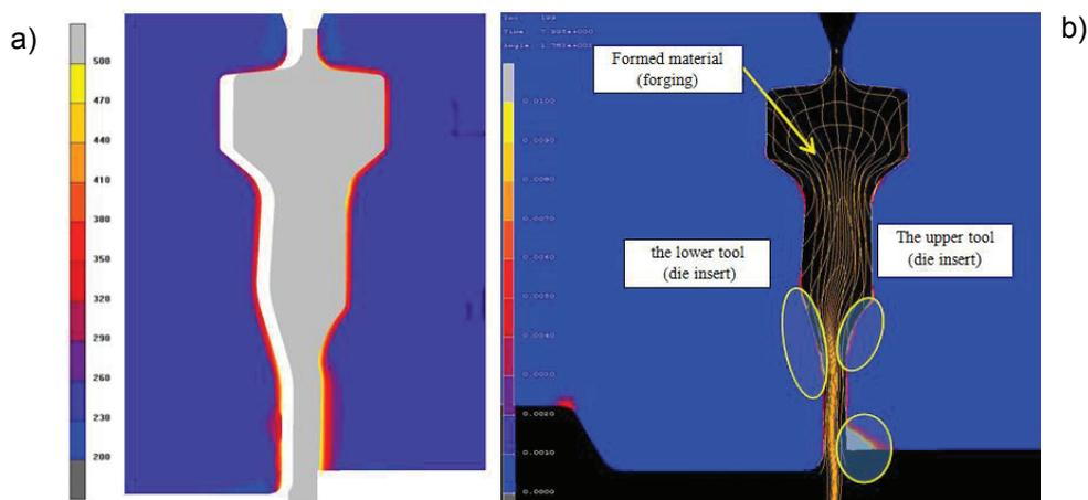
**Figure 2** Distributions of: a) temperature and b) total deformation, obtained from MES (axisymmetrical model) for die inserts made of WCLV preliminarily heated to 250 °C, forging material QS19-20, preform heated to 1150 °C
