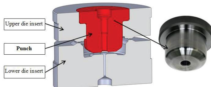
**Figure 3** Tool set in 2nd operation of roughing (preliminary forging)
