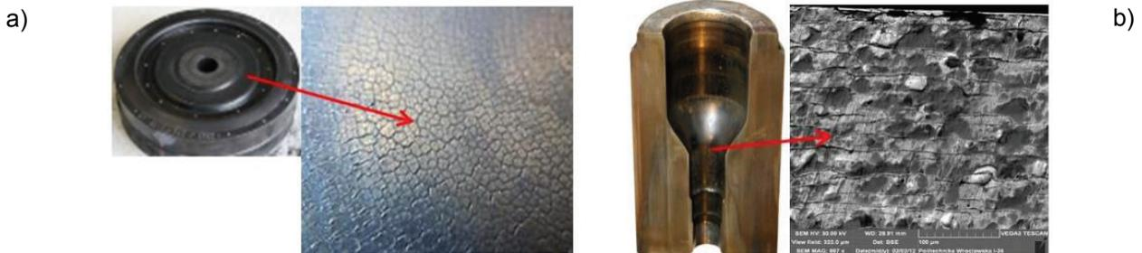
**Figure 1** The view of: a) die after forging of 7900 face wheel forgings with a photograph of the surface, b) die (cut in half) after forging of 8371 CVJB forgings with a SEM photograph of the surface
