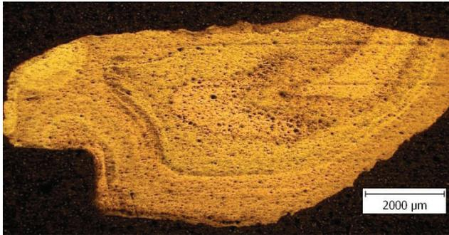
**Figure 6** Dezincification- all cross section, spec. 4
