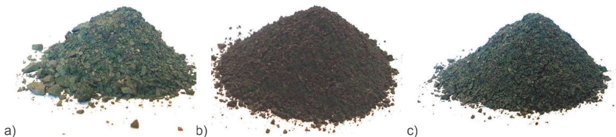
Figure 1 Neodymium magnets recovered from electric motors and powder after melting in three different times: a) 10 s, b) 15 s, c) 30 s
