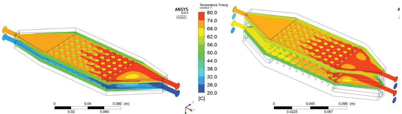
**Figure 3** Heat side of the heat exchangers geometry 3, 4
