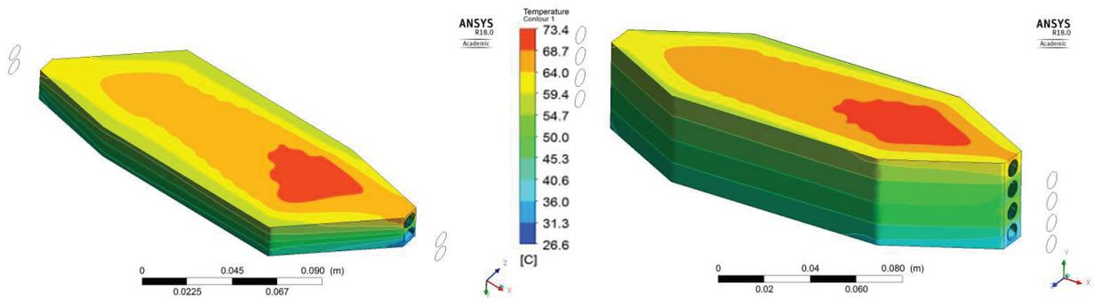
**Figure 5** Thermal distribution on the surface geometry 3, 4
