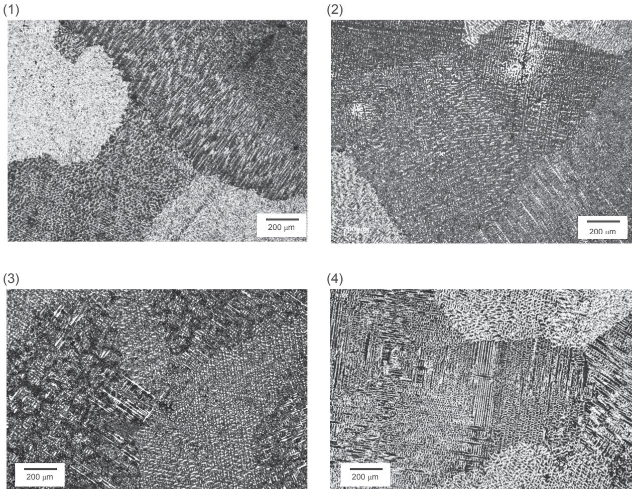
**Figure 2** The microstructure images of dental alloys Remanium CSe ( $\text{Ni}_{61}\text{Cr}_{26}\text{Mo}_{11}\text{Si}_{1.5}$  with a low contents of Fe, Co, Al and Ce) melted and then casted using (1) in flame of oxy-acetylene torch, (2) induction furnace, (3) Volta's arc, (4) in the Autocast device
