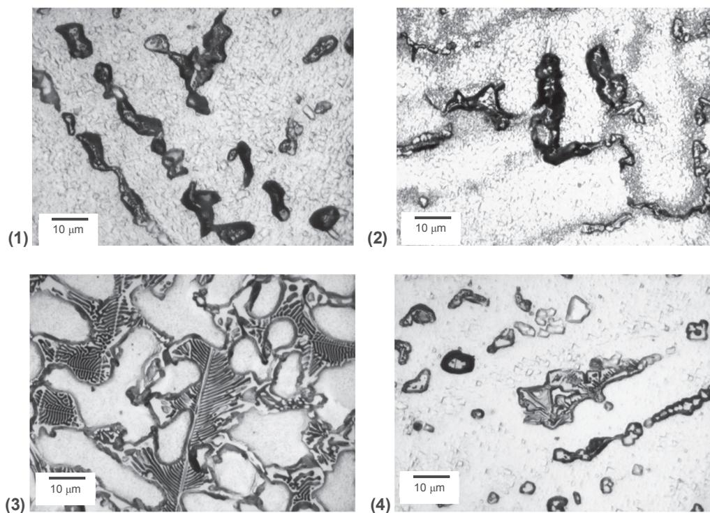
**Figure 4** The microstructure images of dental alloys Remanium CSe ( $\text{Ni}_{61}\text{Cr}_{26}\text{Mo}_{11}\text{Si}_{1.5}$  with a low contents of Fe, Co, Al and Ce) melted and then casted using (1) in flame of oxy-acetylene torch, (2) induction furnace, (3) Volta's arc, (4) in the Autocast device
