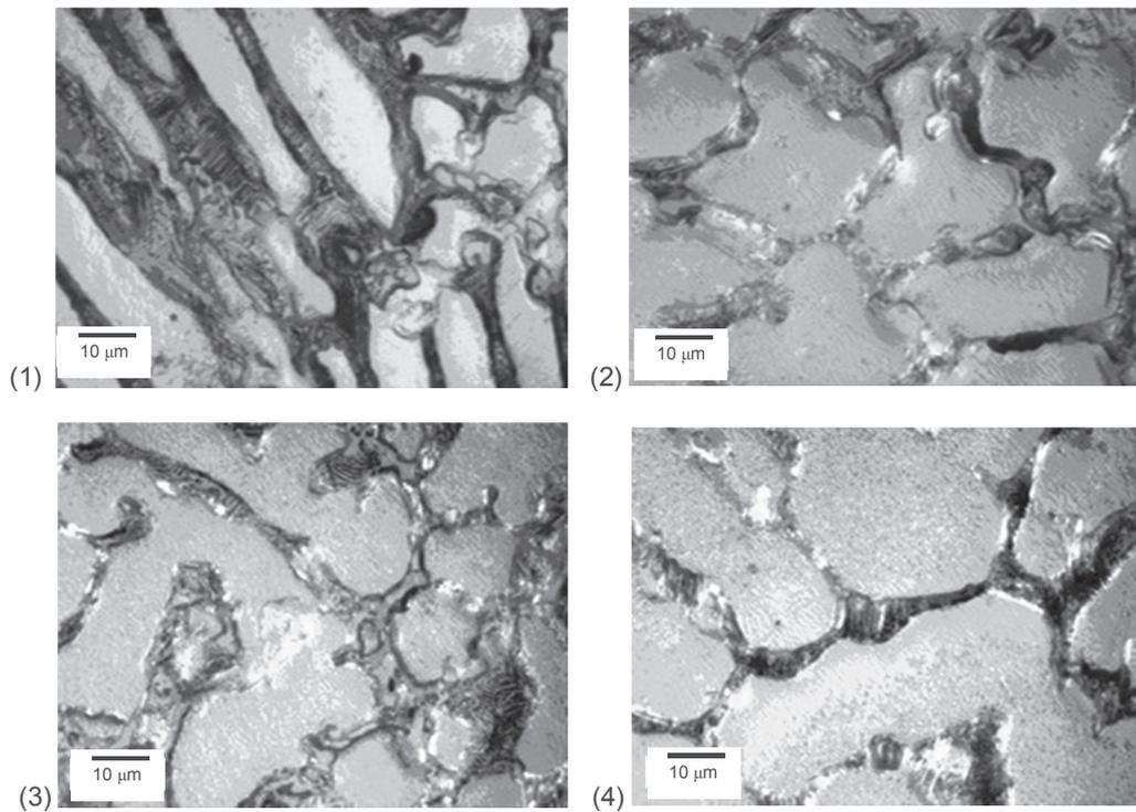
**Figure 3** The microstructure images of dental alloys Remanium G ( $\text{Ni}_{66}\text{Cr}_{27}\text{Mo}_5\text{Si}_2$  with low content of Mn and B) melted and then casted using (1) in flame of oxy-acetylene torch, (2) induction furnace, (3) Volta's arc, (4) in the Autocast device
