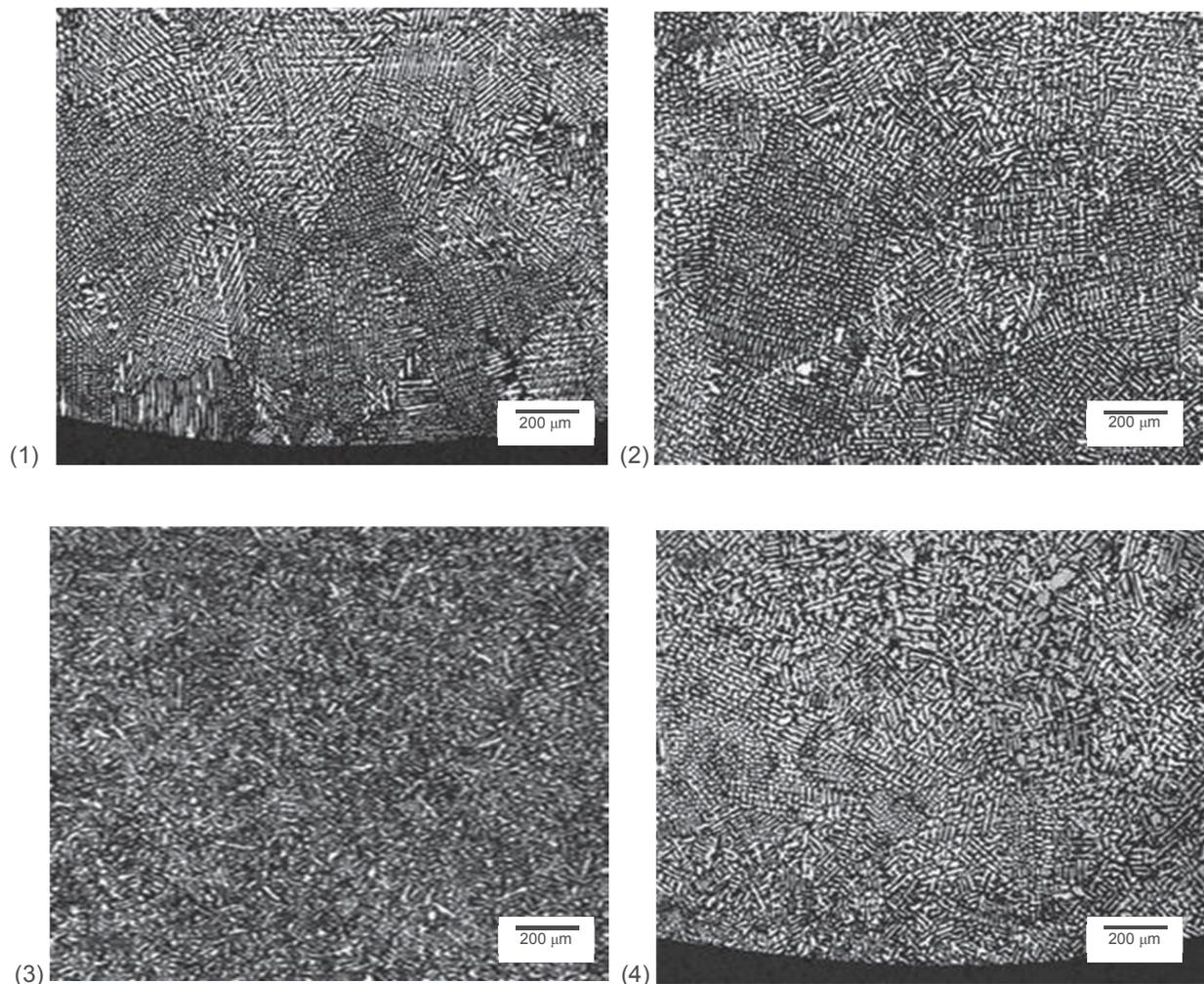
**Figure 1** The microstructure images of dental alloys Remanium G ( $Ni_{66}Cr_{27}Mo_5Si_2$  with low content of Mn and B) melted and then casted using (1) in flame of oxy-acetylene torch, (2) induction furnace, (3) Volta's arc, (4) in the Autocast device
