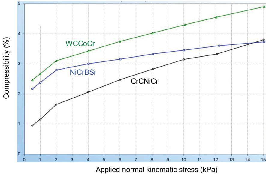
**Figure 5** Compressibility 0.5 - 15 kPa of CrCNiCr, NiCrBSi, and WCCoCr powders
