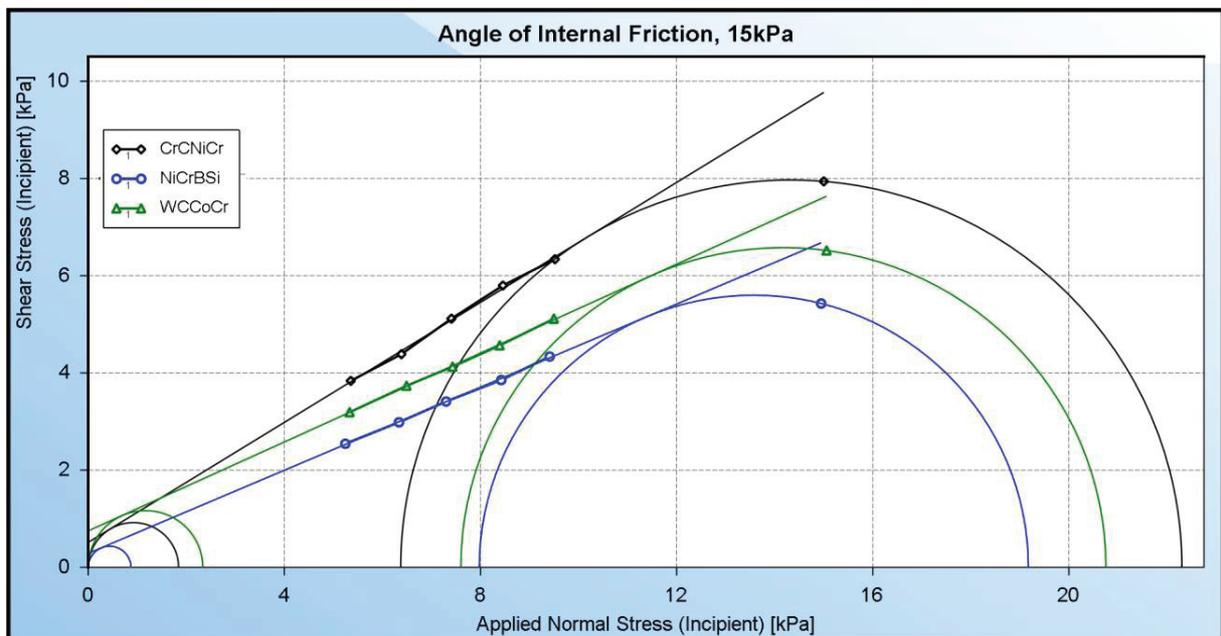
**Figure 4** Angle of internal friction comparison at 15 kPa
