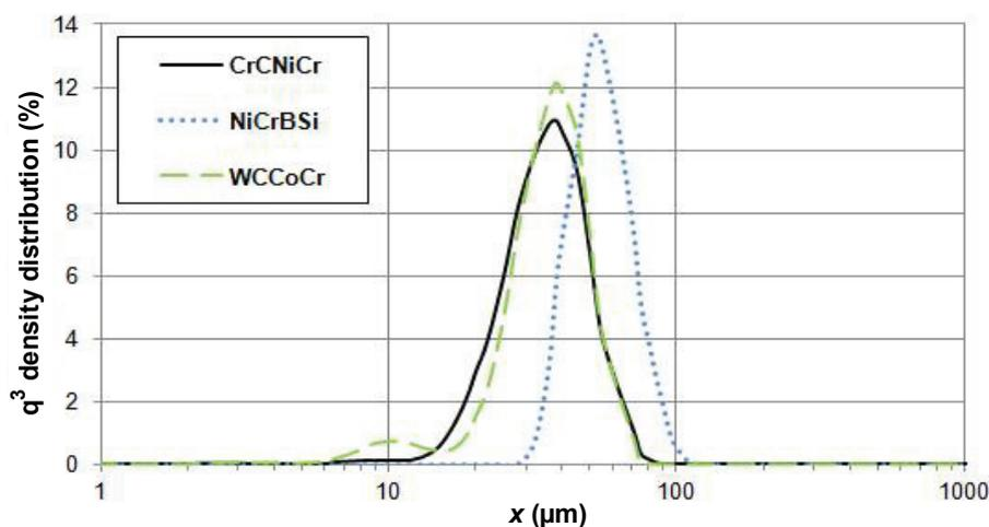
**Figure 2** Particle size distribution of CrCNIr, NiCrBSi, and WCCoCr powders
