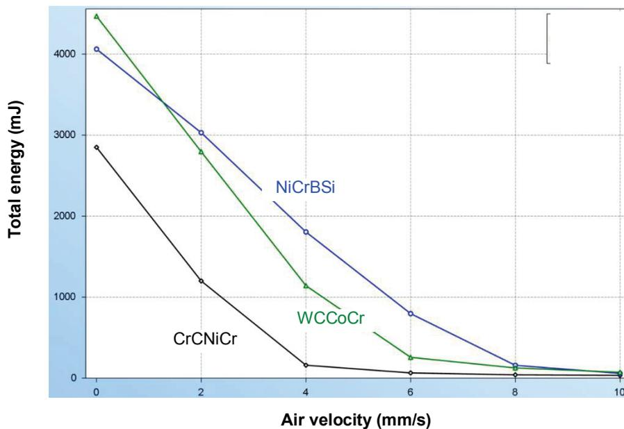
**Figure 6** Aeration test at 0 - 10 mm/s of CrCNiCr, NiCrBSi, and WCCoCr
