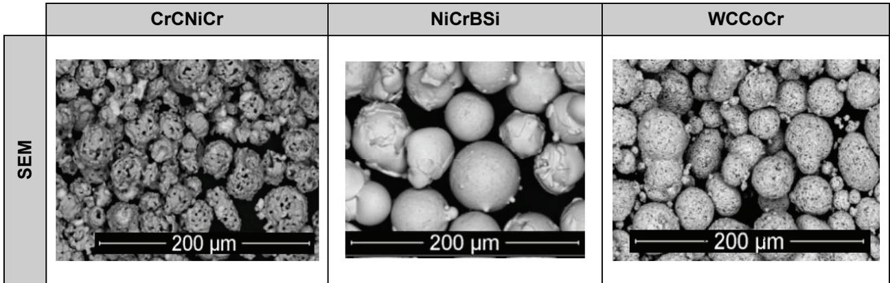
**Figure 3** SEM images of CrCNiCr, NiCrBSi, WCCoCr powder particles
