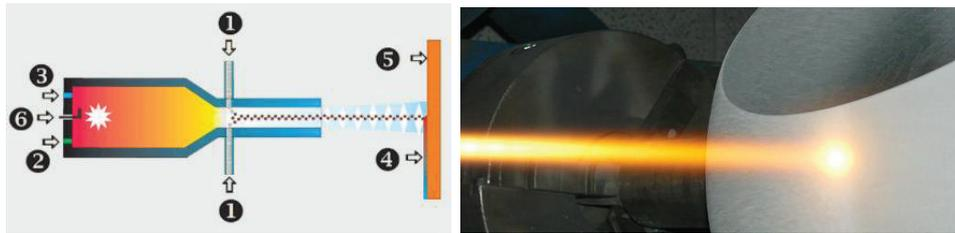
**Figure 1** Basic principle of HVOF technology and its practical application [2]
