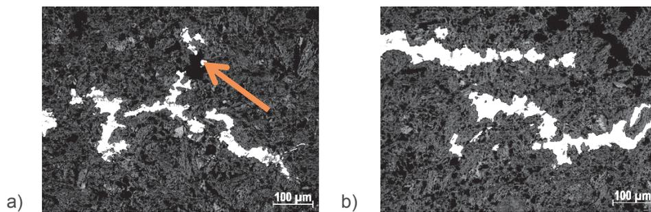
**Figure 6** Microstructure of C sample impregnated by melted zinc under pressure of a) 1.5 MPa; b) 3 MPa
