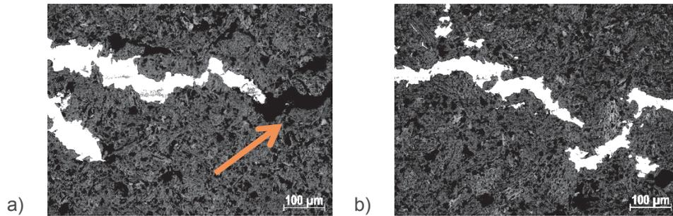
**Figure 5** Microstructure of C sample impregnated by melted tin under pressure of a) 1.5 MPa; b) 3 MPa
