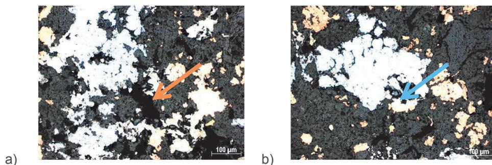
**Figure 8** Microstructure of C/Cu sample impregnated by melted zinc under pressure of a) 1.5 MPa; b) 3 MPa
