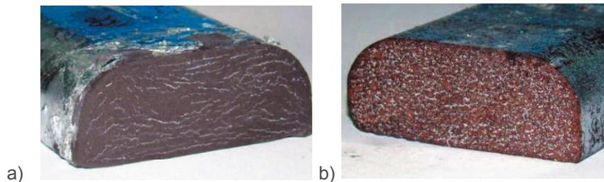
**Figure 2** Macrographs of samples impregnated using melted zinc a) C and b) C/Cu
