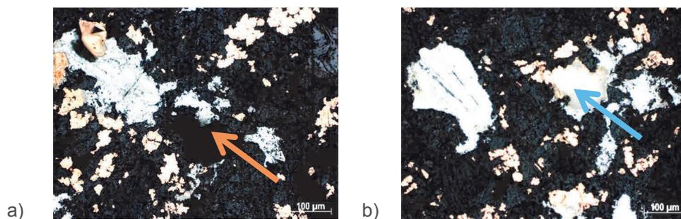
**Figure 7** Microstructure of C/Cu sample impregnated by melted tin under pressure of a) 1.5 MPa; b) 3 MPa
