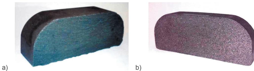
**Figure 1** Macrographs of sintered a) C and b) C/Cu samples
