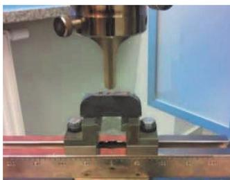
**Figure 3** Bending strength test
